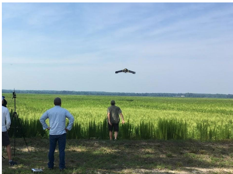
Figure 11.5. Fixed wing eBee Plus drone used in marsh vegetation surveys. Image credit: A. Demeo.
