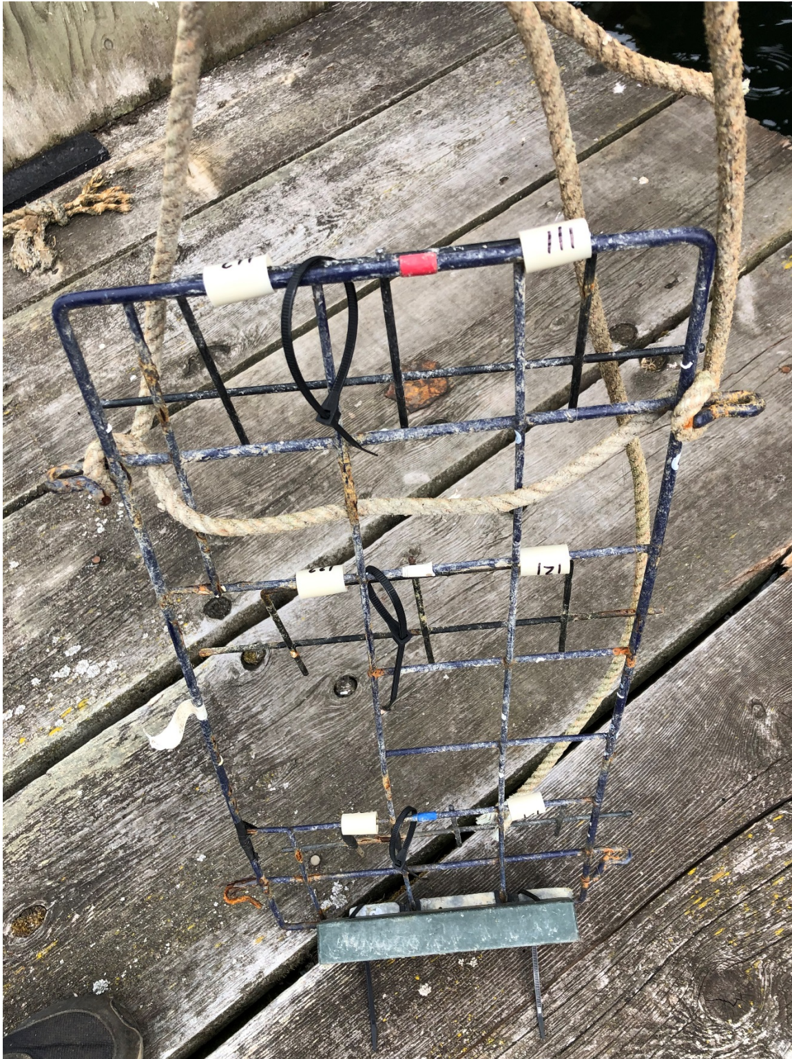
Figure 4. Image of pot panel prior to deployment, equipped with 6 bio-hinges, loosely placed zipties to prevent debris, and a lead weight to keep the soaking gear in place.
