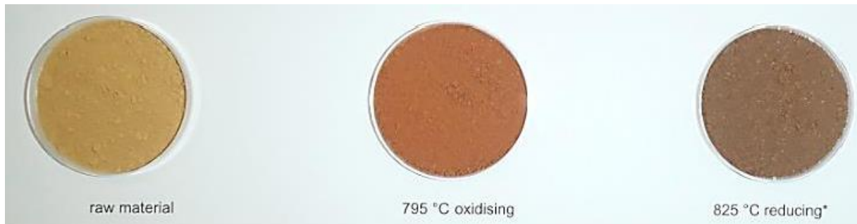
Figure 6-5: Influencing the product colour by varying the calcination conditions of the kaolinitic AWS sample from Rennes/France (SL-2020-06-CH)
