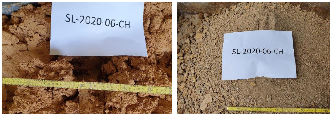
Figure 5-14: Kaolinitic AWS (SL-2020-06-CH) before (left) and after drying (right)
