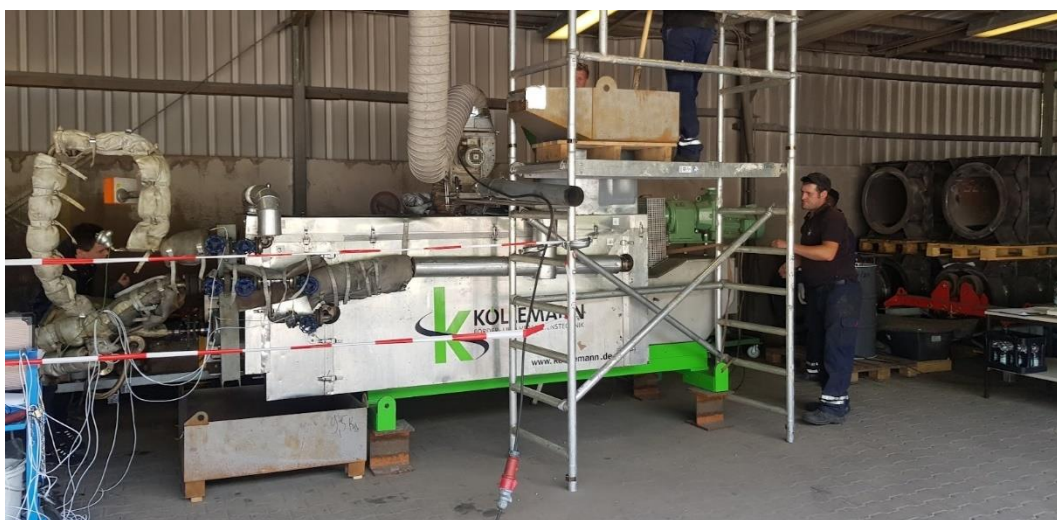
Figure 5-10: Koellermann testing facility with drying screw
