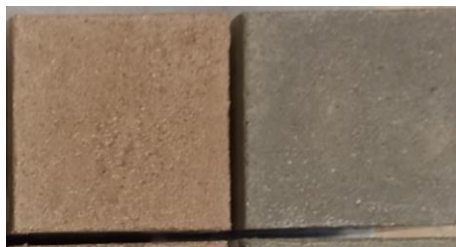
Figure 6-6: Examples of concrete colour in calcined clay cements. Left, calcination under oxidizing conditions; right, calcination under reducing conditions
