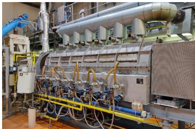
Figure 5-16: IBU-tec testing kiln installation (IBU-tec, 2020)
