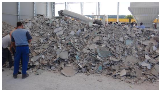
Figure 3-5: DCS in a construction waste recycling plant
