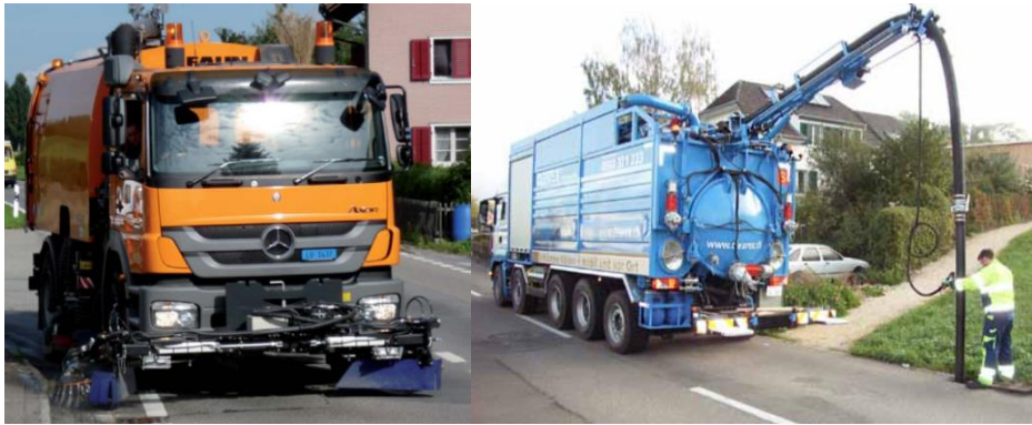
Figure 3-4: Left: Road cleaning truck (Kanton Luzern, 2013); Right: cleaning of road drainage (Cahans, 2017)
