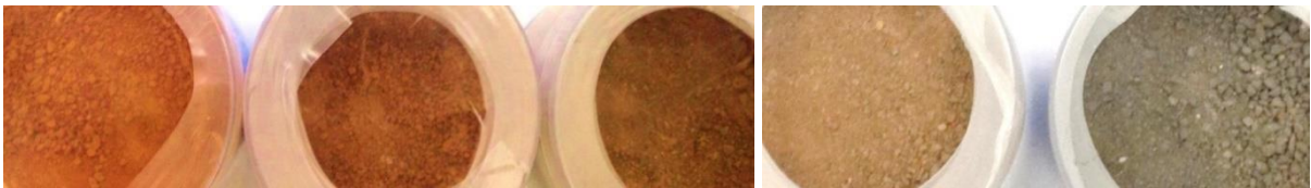
Figure 3-7: Tests conducted with different oxygen levels from (left) fully oxidizing to (right) reducing conditions
