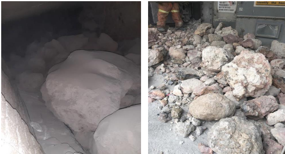
Figure 3-9: Formation of mullite balls due to high burning zone temperature in a rotary calciner
