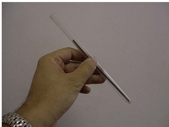
Fig. 7. UNISAT-4 hysteresis rod encapsulated in a vacuum glass tube for thermal treatment.
