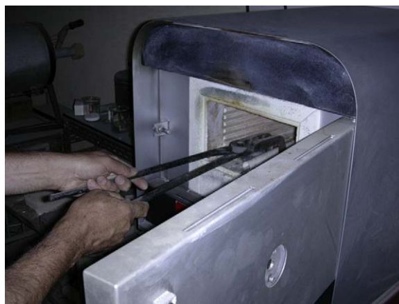
Fig. 8. Thermal treatment of the hysteresis rod in high-temperature oven.
