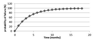
Fig. 1 — Relationship over long runs between failure probability and time
