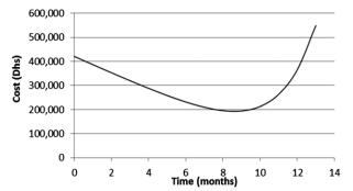
Fig. 3 — Total maintenance expenses as a function of time since the last maintenance
