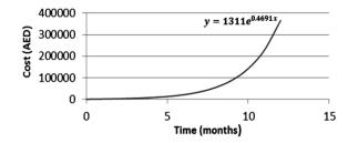
Fig. 5 — Estimated maintenance costs based on the interval since the last maintenance
