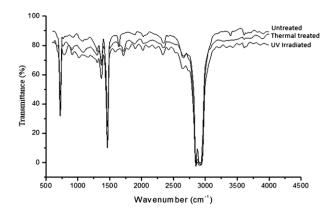
Fig. 1 — FTIR spectra of untreated LDPE films, thermally treated LDPE films at 70°C for 144 h and photo-oxidized (UV irradiated) LDPE films for 144 h
