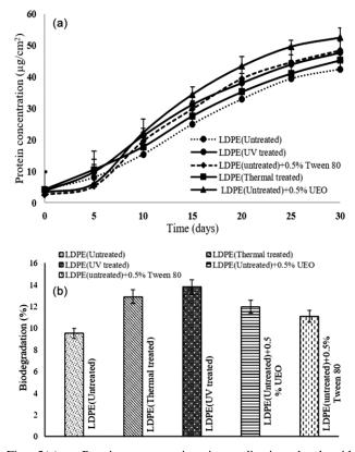
Fig. 2(a)— Protein concentration in media inoculated with *L. fusiformis* TPB using untreated, thermal and UV pretreated LDPE and effect of 0.50% Tween 80 and UEO on biofilm formation (b) Biodegradation of untreated and pretreated LDPE films in mineral salt media by isolated *L. fusiformis* TPB in 30 days
