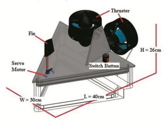
Fig. 2 — 3D model of underwater robot design
