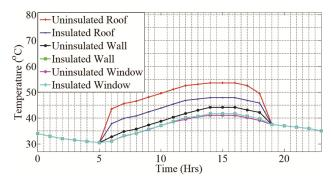
Fig. 3 — Solar air temperature for both test model.
