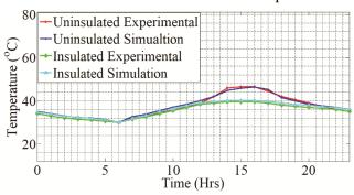
Fig. 8 — Simulated and experimental indoor temperature for uninsulated and insulated model.
