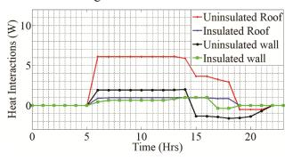
Fig. 4 — Heat interactions from roof and wall oftest model without and with insulation.
