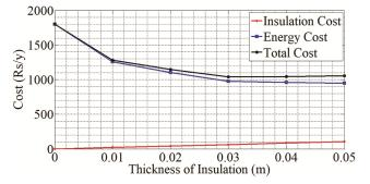
Fig. 9 — Optimum thickness of insulation.
