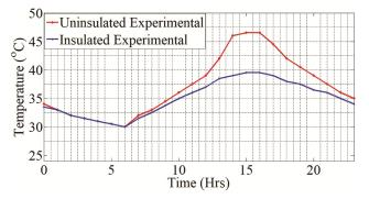
Fig. 7 — Experimental indoor temperature for insulated and uninsulated model.
