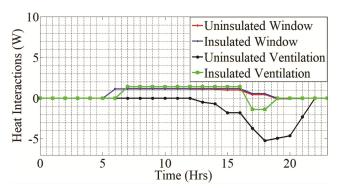
Fig. 5 — Heat interactions from window andventilation for insulated and uninsulated model
