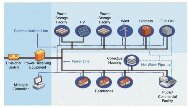
Figure 6. Typical scheme of a micro-grid [40].
