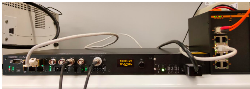
Fig. 3.8 Meinberg microSync NTP/PTP Time Source.
