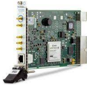
Fig. 3.9 National Instrument NI 6683H timing and synchronization module.
