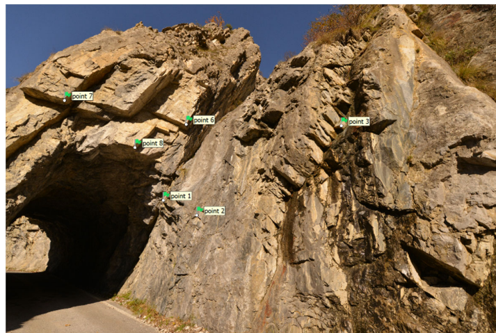
Figure 10. Examples of natural markers used for georeferencing the specific DSMs.
