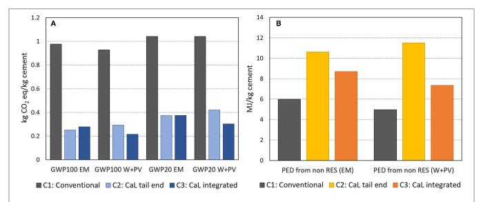
FIGURE 7 | Sensitivity analysis. (A) GWP100 and GWP20 of the systems analyzed per kg of cement produced related to the scenario of the present (Ecoinvent, 2020) electricity production mix (EM) and to a scenario dominated by renewable energy resources (RES), i.e., 50% wind and 50% photovoltaics (W+PV). (B) Primary energy demand (PED) from non-renewables resources (non-RES) related to the same two different scenarios, i.e., EM and W+PV.
