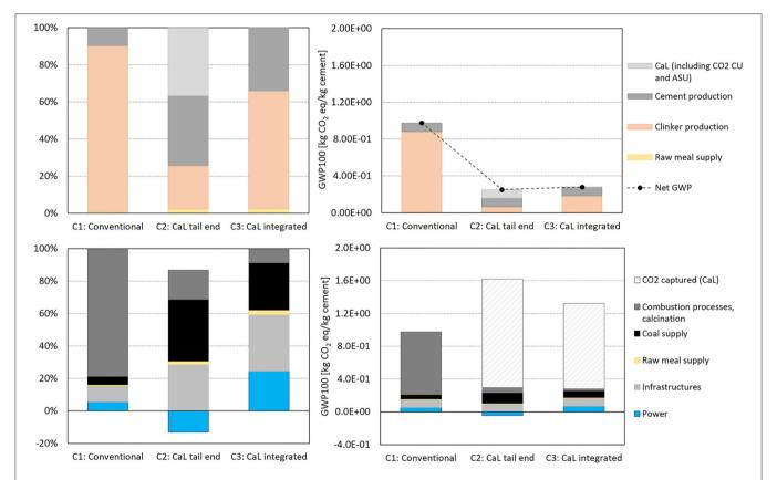
FIGURE 5 | GWP100 contribution analysis and relative emissions of the systems analyzed per kg of cement produced by the different phases (upper panels) and type of processes (lower panels) of the entire cement production cycle.
