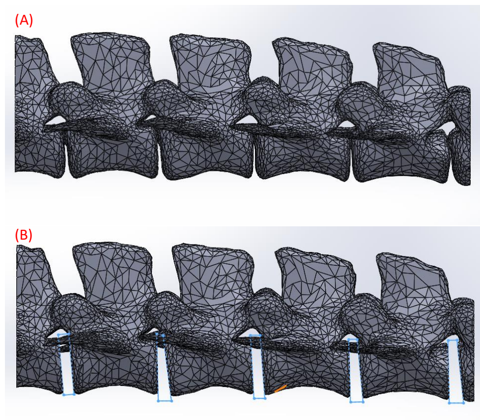
Figure 7.5: A) Basic model CAD on import and B) slices made to separate model into bodies.
