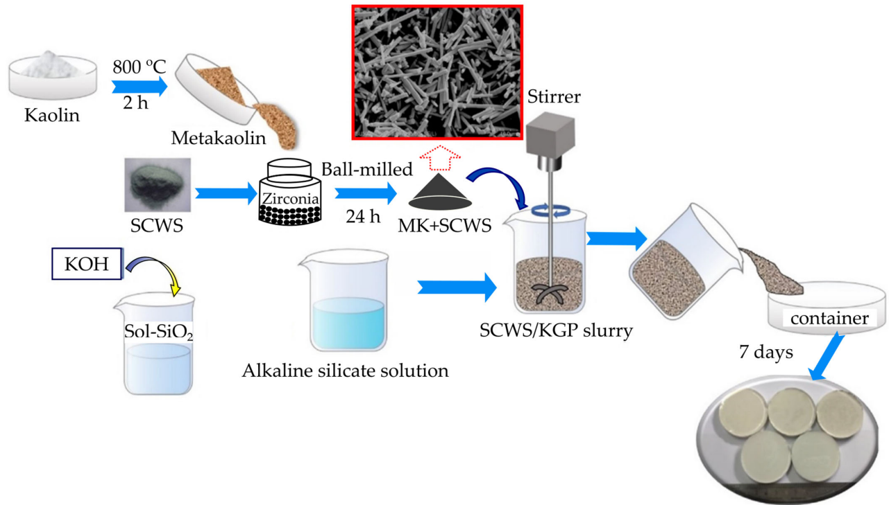
Figure 2. Preparation procedure for SCWS (SiC whiskers)/KGP (Kaolin Geopolymer) composite [46].
