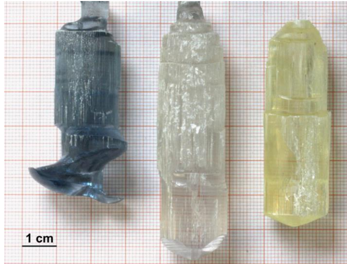
Figure 1.9 \beta -Ga 2 O 3 single crystals obtained by the Czochralski method showing a transition from a spiral to a straight cylinder shape by lowering the free electron concentration from 2 \times 10^{18} \text{ cm}^{-3} (left) to 4 \times 10^{16} \text{ cm}^{-3} (middle) and to insulating state by doping with Mg (right) [56].
