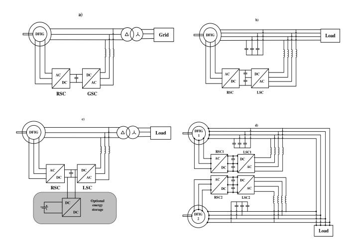
**Fig. 1.1.** Basic DFIG topologies: a) grid-connected DFIG, b) 4-wire stand-alone DFIG, c) 3wire stand-alone DFIG with an intermediate transformer, d) parallel operating DFIGs in a microgrid.
