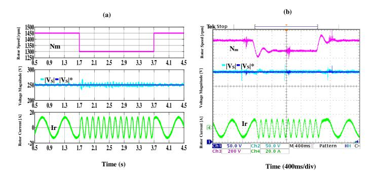
**Fig 3.15** FS-PCC system response under rotor speed variety .a Simulation results .b Experimental. CH1: rotor speed (200 rpm/div), CH2: reference of stator voltage amplitude (50V/div), CH3: stator voltage magnitude (50V/div), CH4: rotor phase current (20A/div).
