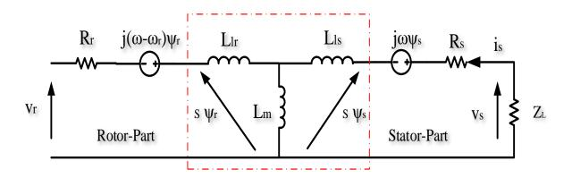
Fig. 2.4. Equivalent circuit of DFIG in arbitrary reference frame by rotation speed of  $\omega$ .
