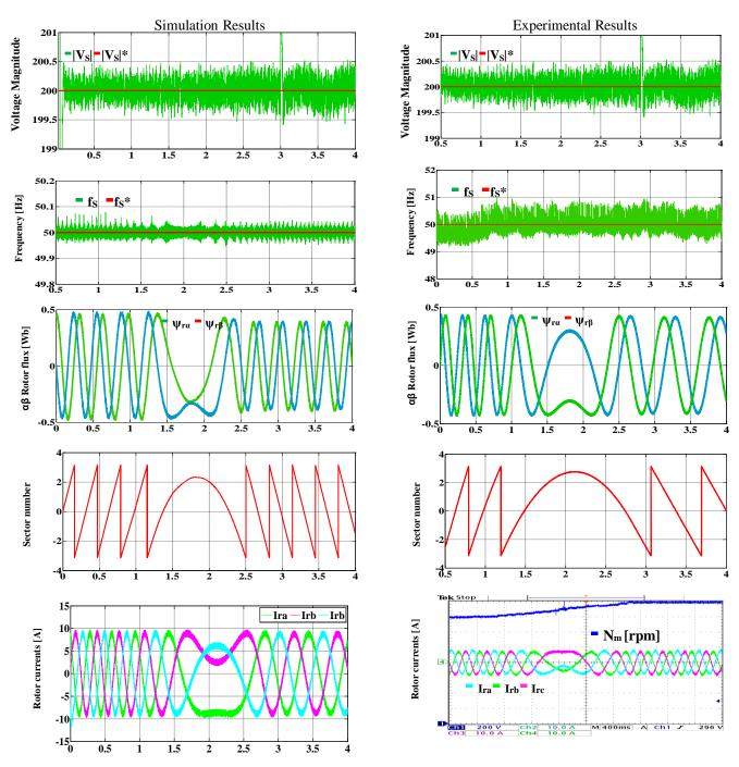
**Fig. 4.12.** Rotor speed change test with the standalone-DFIG operating at fixed Voltage-reference. From top to bottom: Stator voltage magnitude, stator frequency, rotor flux, electromagnetic torque, slip angle, and rotor current waveform. (Left) Simulation results. (Right) Experimental test.
