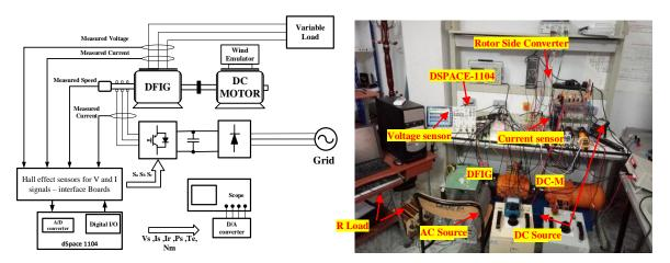
Fig. 3.4 A laboratory prototype of the experimental setup.
