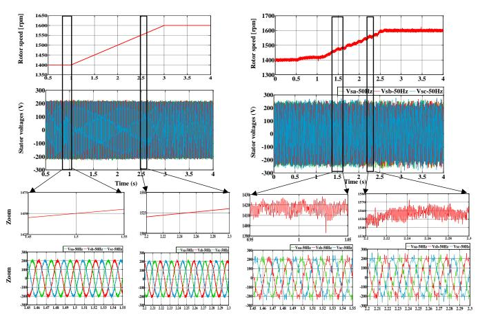
Fig. 4.13. Three phase stator voltage-waveforms during rotor speed change. From top to bottom: Stator voltage magnitude, stator frequency, rotor flux, stator current waveform. (Left) Simulation results. (Right) Experimental test.
