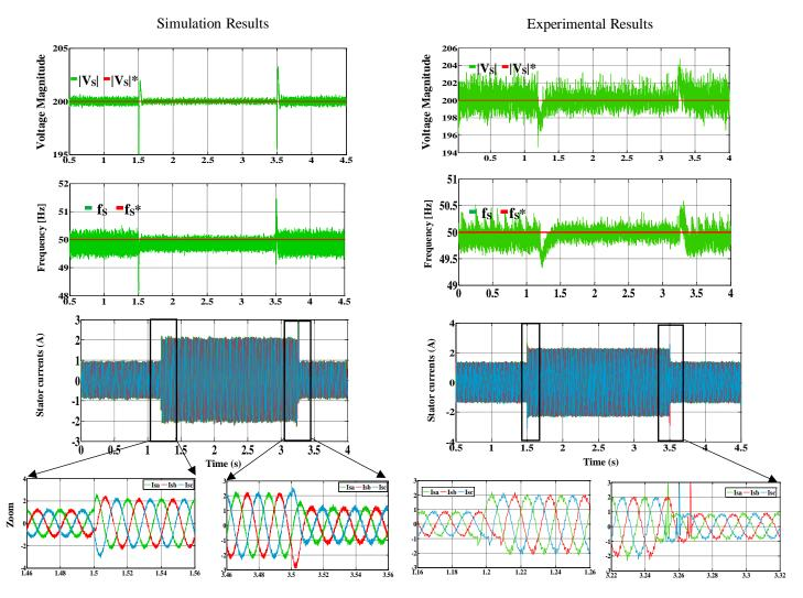
Fig. 4.11. Three phase stator currents-waveforms during load change. From top to bottom: Stator voltage magnitude, stator frequency, stator voltage waveform. (Left) Simulation results. (Right) Experimental test.
