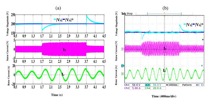
**Fig. 3.7** HCC system response under load variety a Simulation results b Experimental. CH1: reference of stator voltage magnitude (50V/div), CH2: stator voltage magnitude (50V/div), CH3: stator phase current (5A/div), CH4: rotor phase current (20A/div).
