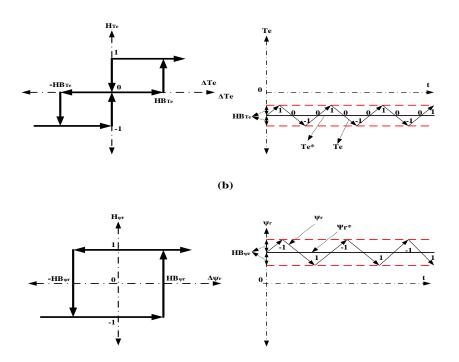
Fig. 4.6. (a) Three-level hysteresis comparator for the torque control,(b) Two-level hysteresis comparator for flux control.
