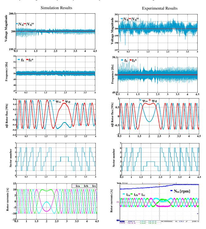
**Fig. 4.18.** Rotor speed change test with the standalone-DFIG operating at fixed Voltage-reference. From top to bottom: Stator voltage magnitude, stator frequency, rotor flux, electromagnetic torque, slip angle, and rotor current waveform. (Left) Simulation results. (Right) Experimental test.
