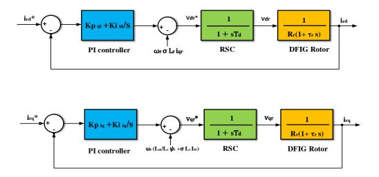
Fig. 2.8. Closed-loop system of the *d*-*q* axis current control [66].
