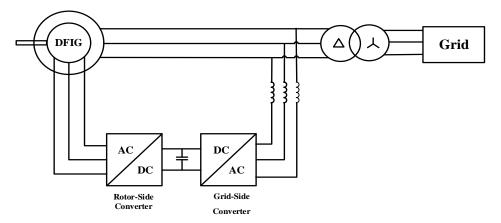
Fig. 2. Parallel topology of the grid-connected generator.
