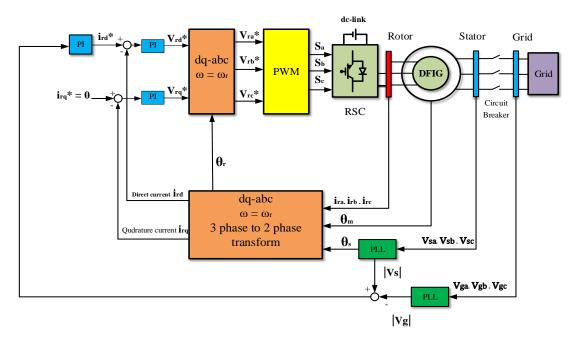
Fig. 1.7. Diagram block for FOC-based synchronization process.
