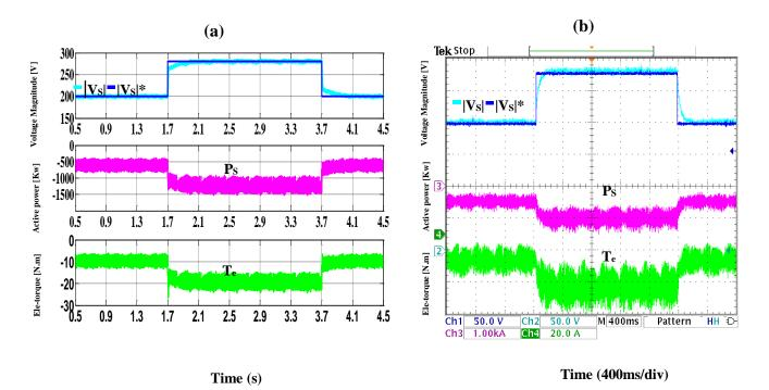
**Fig. 3.11** FS-PCC system response under step variation in the reference of stator voltage amplitude .a Simulation results .b Experimental.CH1: reference of stator voltage magnitude (50V/div), CH2: stator voltage magnitude (50V/div), CH3: stator active power (1KW/div), CH4: electromagnetic torque (20N.m/div).
