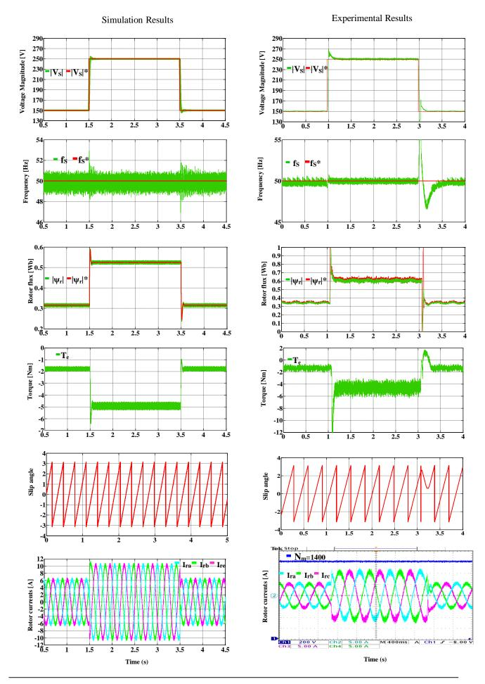
**Fig. 4.8.** Voltage-reference change test with the standalone-DFIG operating at fixed-load. From top to bottom: Stator voltage magnitude, stator frequency, rotor flux, electromagnetic torque, slip angle, and rotor current waveform. (Left) Simulation results. (Right) Experimental test.
