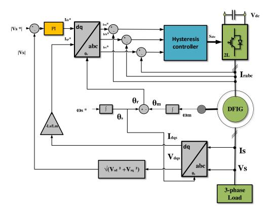
Fig. 3.2. Block diagram of the HCC for RSC.
