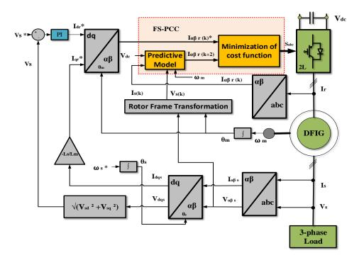
Fig. 3.3 Block diagram of FS-PCC for RSC.
