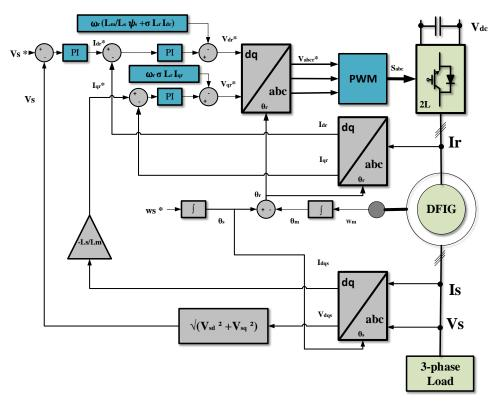
Fig. 2.7. Basic control strategy scheme of the RSC for stand-alone DFIG system.
