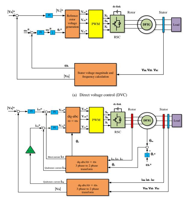
(b) Indirect stator flux oriented (ISFO)
