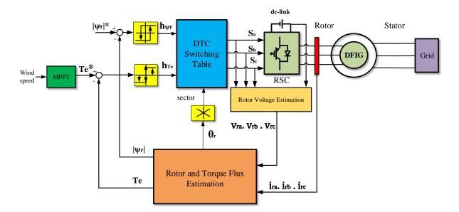
Fig. 1.4. Typical block diagram of direct torque control (DTC).
