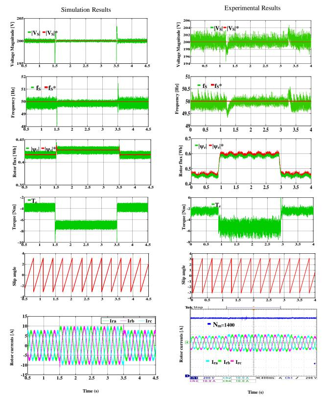
**Fig. 4.10.** Load change test with the standalone-DFIG operating at fixed Voltage-reference. From top to bottom: Stator voltage magnitude, stator frequency, rotor flux, electromagnetic torque, slip angle, and rotor current waveform. (Left) Simulation results. (Right) Experimental test.
