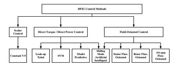
Fig. 1.2. Classification of DFIG control methods.
