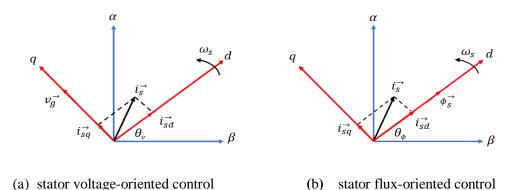
Fig 2.5 Vector diagram of the DFIG control system.
