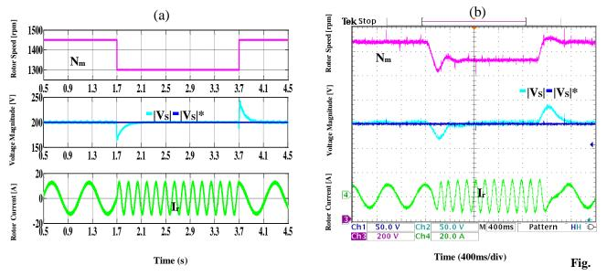
**3.8** HCC system response under rotor speed variety. CH1: rotor speed (200 rpm/div), CH2: reference of stator voltage magnitude (50V/div), CH3: stator voltage magnitude (50V/div), CH4: rotor phase current (20A/div).
