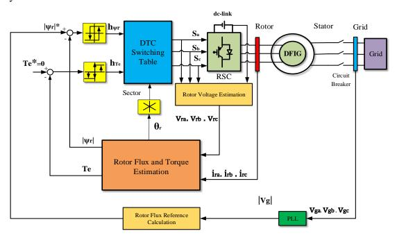
Fig. 1.8. Diagram block for DTC for DFIG grid synchronization.
