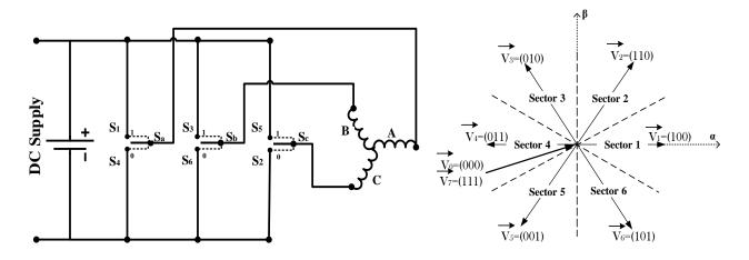
Fig. 4.7. RSC switching positions and voltage switching vectors.
