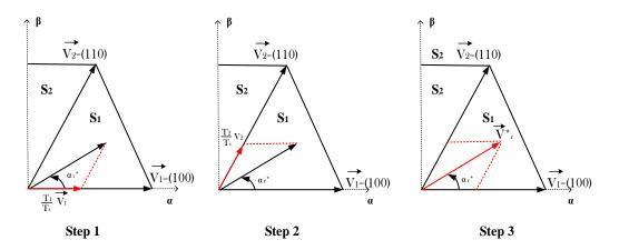
Fig. 4.3 Modulation algorithm steps.
