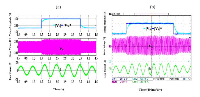
**Fig. 3.5** HCC system response under step variation in the reference of stator voltage amplitude .a Simulation results .b Experimental.CH1: reference of stator voltage magnitude (50V/div), CH2: stator voltage magnitude (50V/div), CH3: stator phase voltage (200V/div), CH4: rotor phase current (20A/div).
