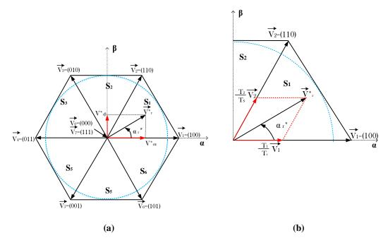
**Fig. 4.2.** (a) Basic switching vectors and sectors. (b) Projection of the reference voltage vector on two adjacent vectors.
