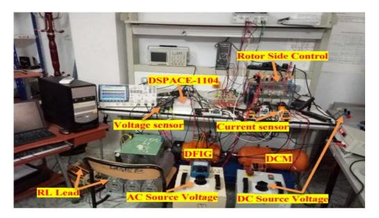
Fig. A.1. Presentation of the experimental setup.
