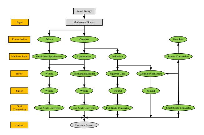
Fig. 4. Technological roadmap for wind turbine's technology [28].
