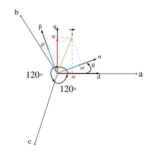
**Fig. 2.3.** State-space two-axis representation of three-phase (a-b-c) systems showing the relationship between the rotor  $(\alpha-\beta)$  and synchronous (d-q) reference frames.
