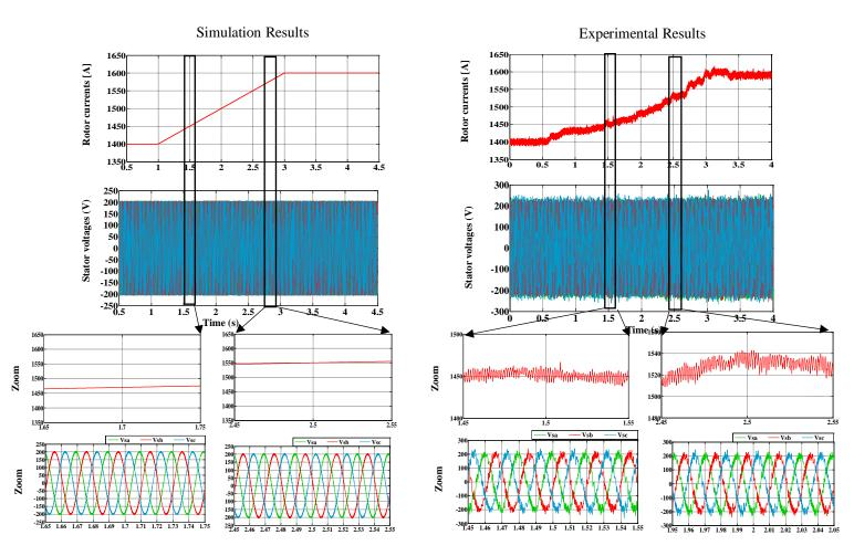
Fig. 4.19. Three phase stator voltage-waveforms during rotor speed change. From top to bottom: Stator voltage magnitude, stator frequency, rotor flux, stator current waveform. (Left) Simulation results. (Right) Experimental test.
