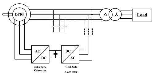
Fig. 3. Parallel topology of the stand-alone generator.
