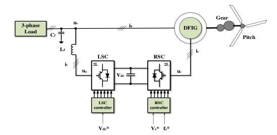
Fig. 2.1 Basic diagram of the standalone WPGSs based on DFIG.
