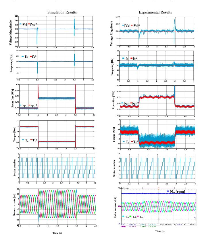
**Fig. 4.16.** Load change test with the standalone-DFIG operating at fixed Voltage-reference. From top to bottom: Stator voltage magnitude, stator frequency, rotor flux, electromagnetic torque, sector number, and rotor current waveform. (Left) Simulation results. (Right) Experimental test.
