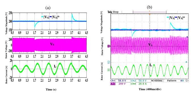
**Fig. 3.6** HCC system response under load variety in the reference of stator voltage amplitude .a Simulation results .b Experimental.CH1: reference of stator voltage magnitude (50V/div), CH2: stator voltage magnitude (50V/div), CH3: stator phase voltage (200V/div), CH4: rotor phase current (20A/div).
