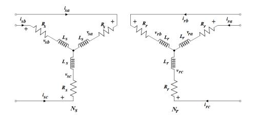
Fig. 2.2. Stator and rotor three-phase circuit of DFIG.
