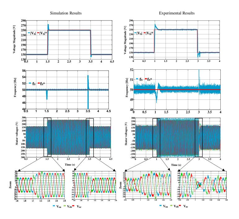
Fig. 4.15. Three phase stator voltage-waveforms during voltage magnitude step change. From top to bottom: Stator voltage magnitude, stator frequency, stator voltage waveform. (Left) Simulation results. (Right) Experimental test.
