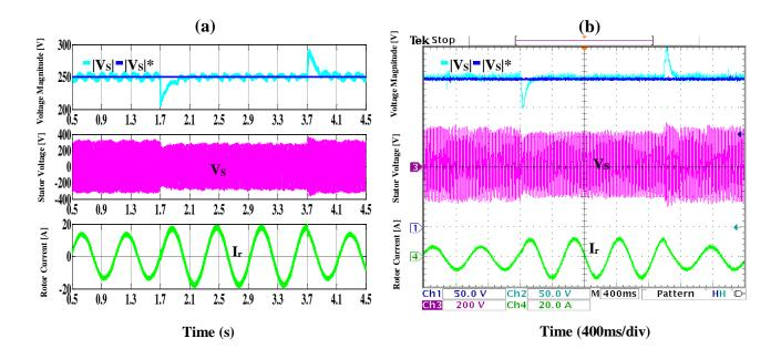
**Fig 3.14** FS-PCC system response under load variety .a Simulation results .b Experimental. CH1: reference of stator voltage magnitude (50V/div), CH2: stator voltage amplitude (50V/div), CH3: stator phase voltage (200V/div), CH4: rotor phase current (20A/div).
