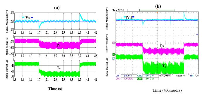
**Fig 3.14** FS-PCC System response under load variety .a Simulation results .b Experimental.CH1: reference of stator voltage magnitude (50V/div), CH2: stator voltage amplitude (50V/div), CH3: stator active power (1KW/div), CH4: electromagnetic torque (20N.m/div).
