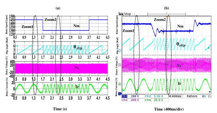
**Fig 3.16** FS-PCC system response under rotor speed variety. a Simulation results .b Experimental. CH1: rotor speed (200 rpm/div), CH2: Slip Angle (5 rad/div), CH3: stator phase voltage (400V/div), CH4: rotor phase current (20A/div).
