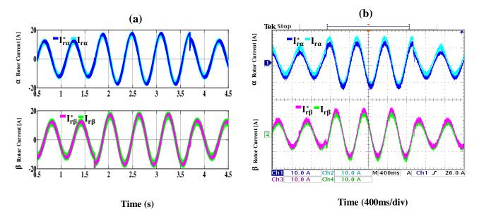
**Fig. 3.10** FS-PCC rotor currents response in  $\alpha\beta$  under stator voltage change .a Simulation results .b Experimental.CH1: reference and measure rotor current in  $\alpha$  axis (10A/div), CH2: reference and measure rotor current in  $\beta$  axis (10A/div).
