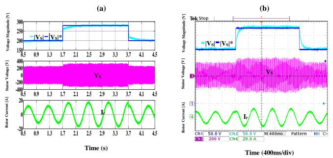
Experimental.CH1: reference of stator voltage magnitude (50V/div), CH2: stator voltage magnitude (50V/div), CH3: stator phase voltage (200V/div), CH4: rotor phase current (20A/div).
