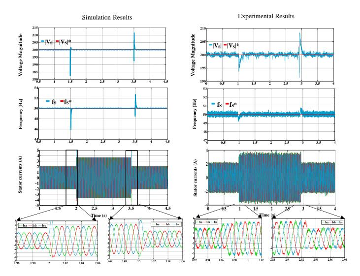
Fig. 4.17. Three phase stator currents-waveforms during load change. From top to bottom: Stator voltage magnitude, stator frequency, stator voltage waveform. (Left) Simulation results. (Right) Experimental test.
