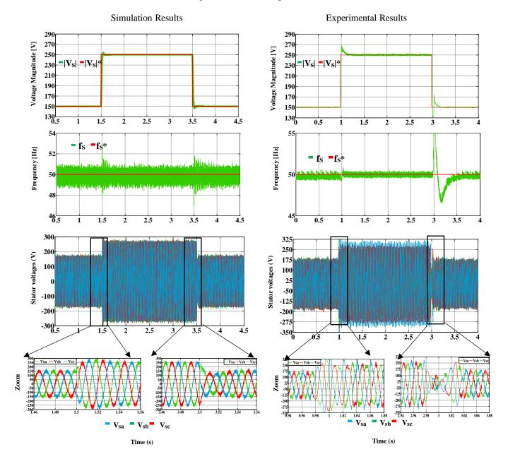
**Fig. 4.9.** Three phase stator voltage-waveforms during voltage magnitude step change. From top to bottom: Stator voltage magnitude, stator frequency, and Stator voltage waveform. (Left) Simulation results. (Right) Experimental test.
