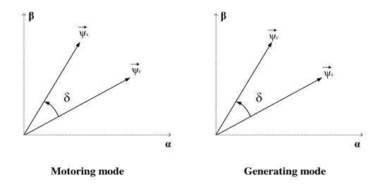
Fig. 4.5. Stator and rotor flux vector at motoring and generating states.
