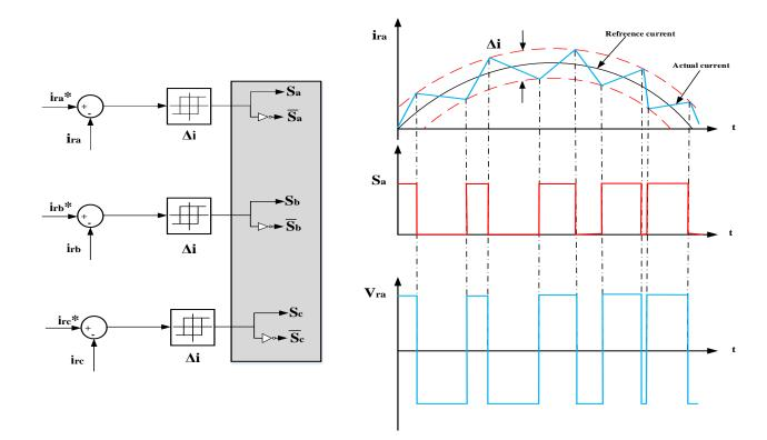
Fig. 3.1. Hysteresis current control operating principles.
