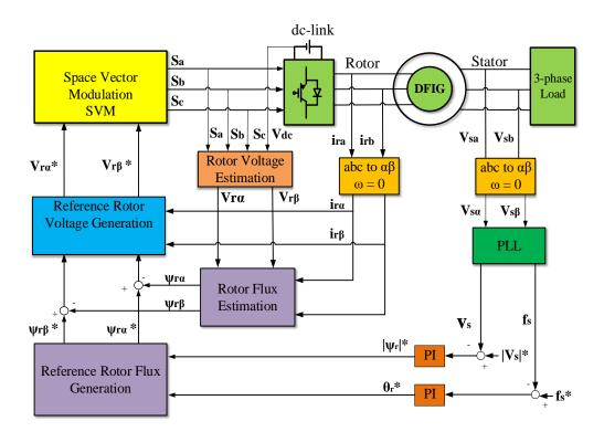
Fig. 4.1. Block diagram of the proposed DRFVC.
