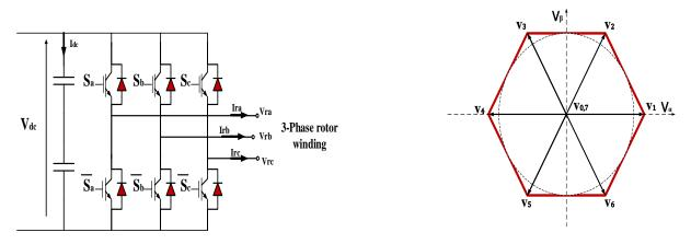
Fig. 2.5. Left: two-level voltage source inverter; right: voltage vectors.
