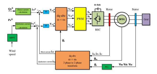
Fig. 1.3. Field oriented control schematic.
