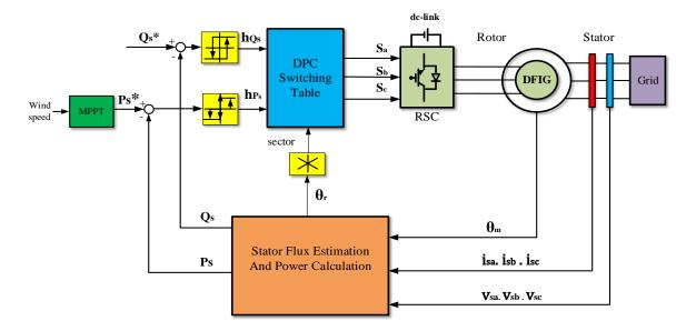
Fig. 1.5. Typical block diagram of direct power control (DPC).
