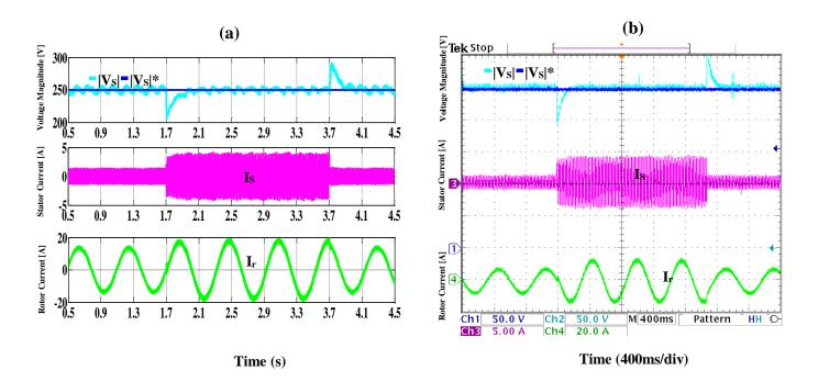
**Fig 3.13** FS-PCC System response under load variety .a Simulation results .b Experimental. CH1: reference of stator voltage magnitude (50V/div), CH2: stator voltage magnitude (50V/div), CH3: stator phase current (5A/div), CH4: rotor phase current (20A/div).
