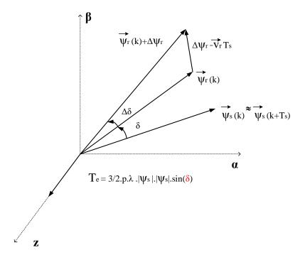
Fig. 4.6. Principles of DTC in  $\alpha\beta$  reference frame.
