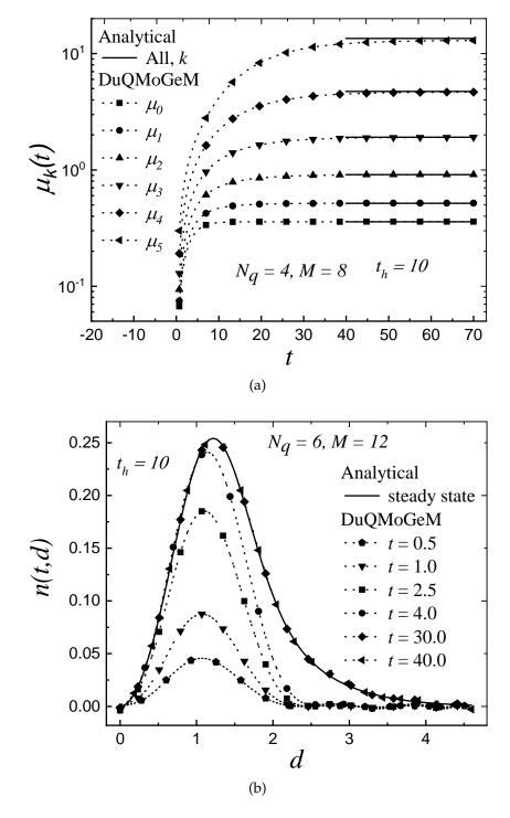
**Figure IV.7:** Pure coalescence problem in a continuous flow extraction vessel: comparison of the analytical and numerical results.
