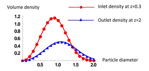
**Figure III.4:** Number density for the pure aggregation by the variational iteration method at z=0.3 (inlet) and z=2.5 (outlet).
