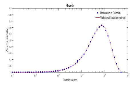
**Figure III.7:** Comparison between the discontinuous Galerkin and Vim for the case of pure growth process.
