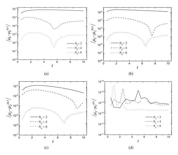
**Figure IV.2:** Pure coalescence problem in a batch extraction vessel: absolute errors for the first four regular moments for the DuQMoGeM solutions with  $N_q = 2, 4$  and 6 using the same number of Gauss-Legendre quadrature points, M = 12.
