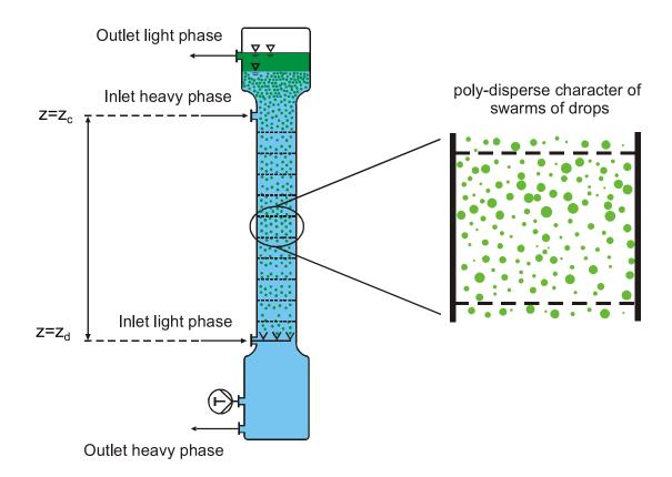
Figure II.1: Schematic of a countercurrent liquid-liquid extraction column Garthe, 2006
