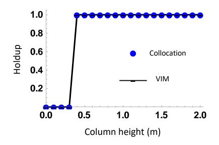
Figure III.3: Holdup versus column height for the pure breakage.
