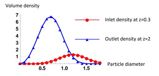
**Figure III.12:** Volume density for the pure breakage with linear velocity by the variational iteration method at z=0.3 (inlet) and z=2.5 (outlet).
