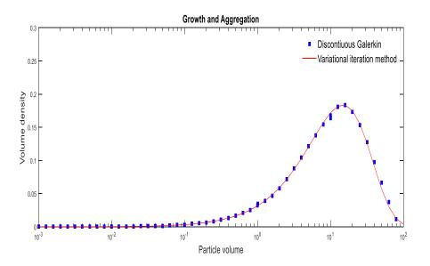
**Figure III.8:** Comparison between the discontinuous Galerkin and Vim for the case of pure growth process.
