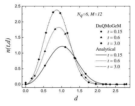
**Figure IV.5:** Simultaneous breakage and coalescence problem in batch extraction vessel: comparison of the analytical and numerical distributions.
