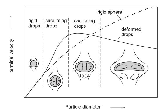
Figure II.4: terminal velocities of single drops and spheres Garthe, 2006
