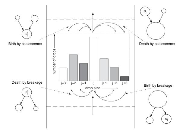
**Figure I.1:** Graphical representation of the breakage and coalescence terms, balance of a drop with diameter  $d_i$  Kopriwa et al., 2012
