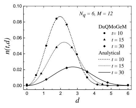
**Figure IV.3:** Pure coalescence problem in a batch extraction vessel: comparison of the analytical and numerical distributions.
