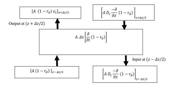
**Figure II.3:** Balance on a reference volume  $A.\Delta z$  for continuous phase.
