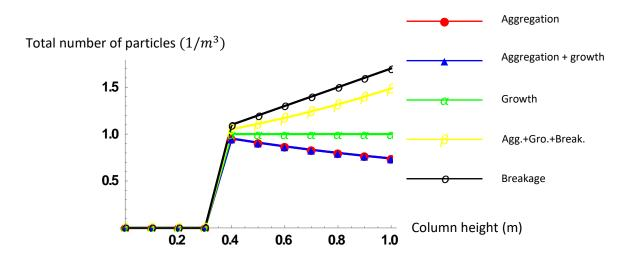
**Figure III.10:** Total number of particles as function of column height for the case of breakage only, aggregation only, growth only, growth + aggregation, and simultaneous all process. Solid lines vim and markers collocation approach
