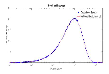
**Figure III.9:** Comparison between the discontinuous Galerkin and Vim for the case of simultaneous growth and breakage process
