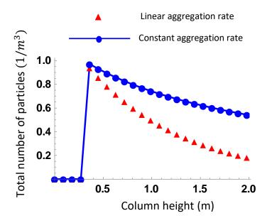
**Figure III.11:** Comparison between the total number of particles versus column height for the case of pure aggregation process with constant aggregation rate and linear aggregation rate.
