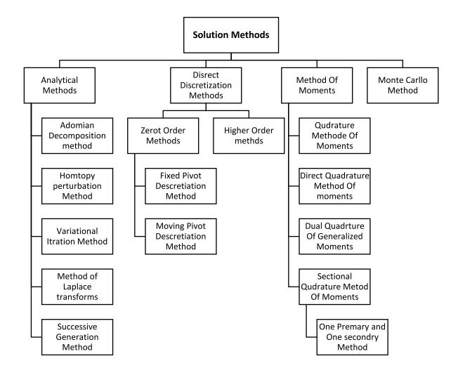
Figure I.2: Numerical and analytical methods to solve the population balance equation
