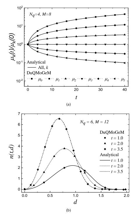
**Figure IV.4:** Pure breakage problem in a batch extraction vessel: comparison of the analytical and numerical results.
