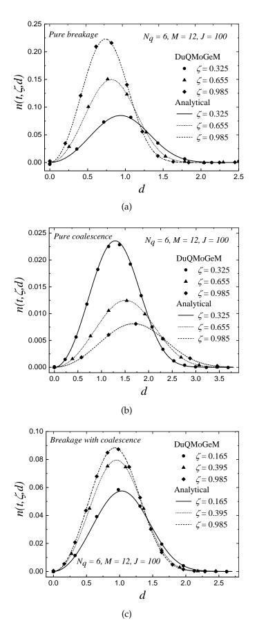
**Figure IV.10:** Comparison of the analytical and numerical distributions in an extraction column.
