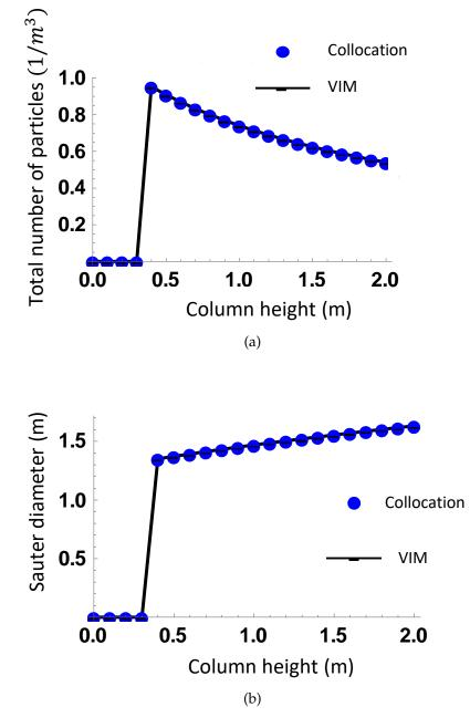
**Figure III.5:** Total number of particles (a), and Sauter diameter (b), as function of column height for the case of pure aggregation process.
