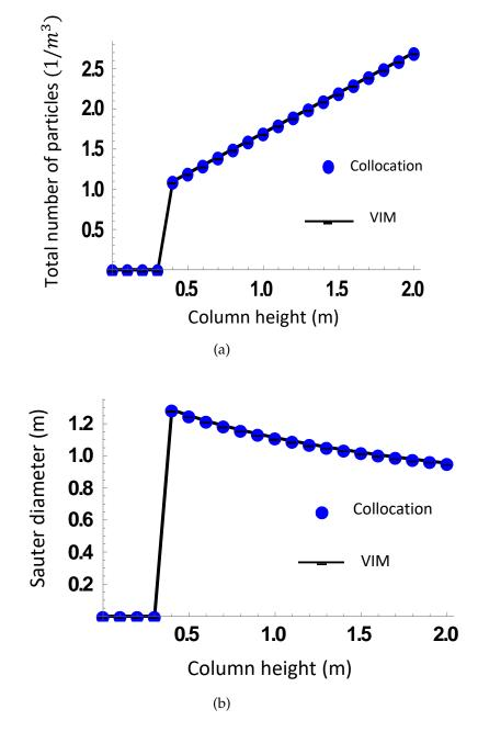
**Figure III.2:** Total number of particles (a), and Sauter diameter (b), as function of column height for the case of pure breakage process.
