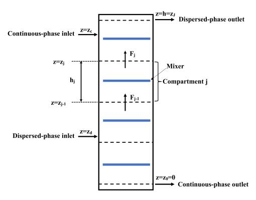
Figure IV.1: Multi-compartment extraction column.
