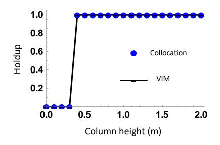
Figure III.6: Holdup versus column height for the pure aggregation.
