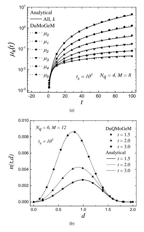
**Figure IV.6:** Pure breakage problem in a continuous flow extraction vessel: comparison of the analytical and numerical results.
