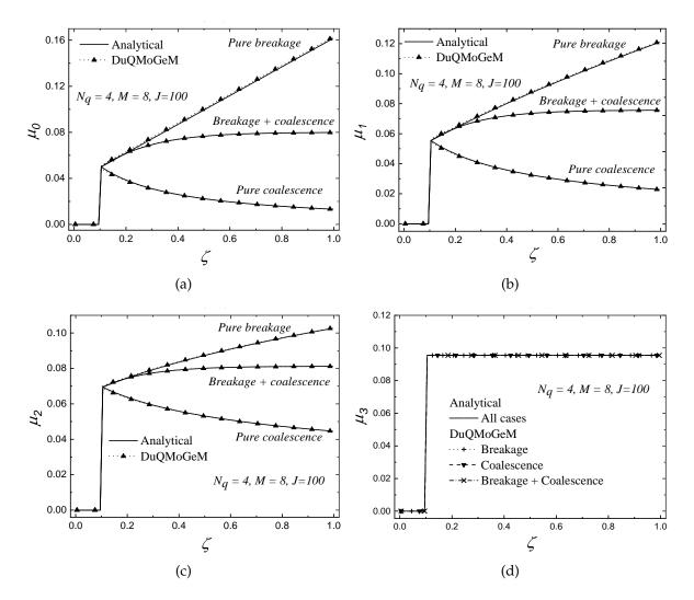
**Figure IV.9:** Comparison of the analytical and numerical moments for steady-state solutions in an extraction column.
