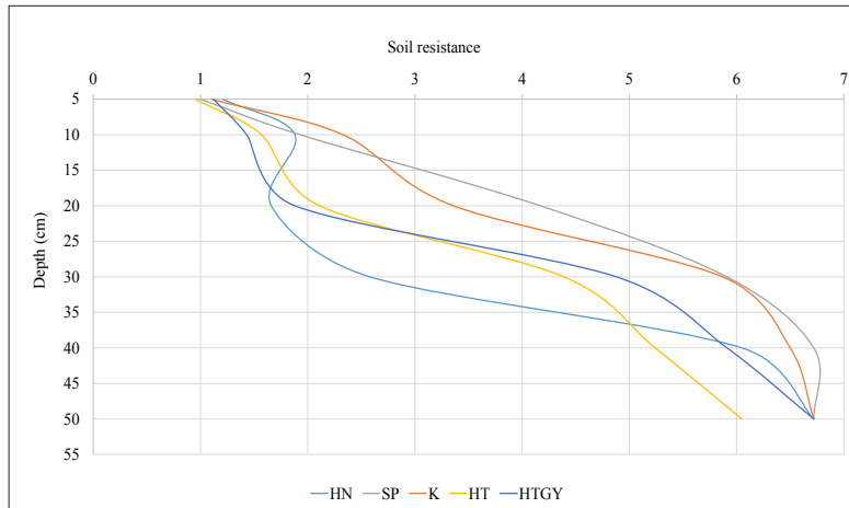
Figure 4. The soil resistance values on the first day of the shallow tillage treatments (Hatvan, 2008.07.13.)
