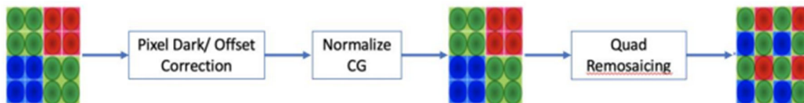
Figure 7: Pixel Calibration Before Remosaicing
