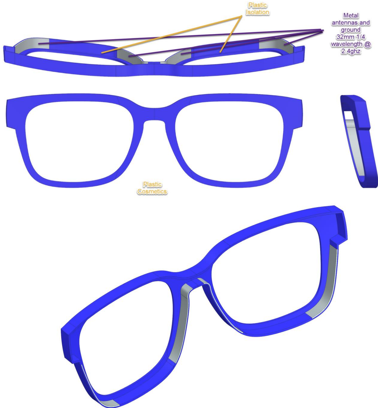
Fig. 3: Another example of front frames acting as antennas. In this case, metal elements (gray) are overmolded on a plastic frame. The structure acts as antennas for RF communication between the glasses and mobile devices or peripherals. The dominant cosmetic or aesthetic element is plastic.
