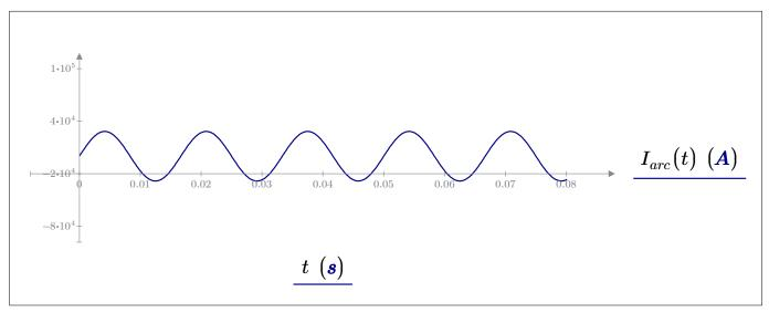
Figure 3. Typical waveform of arc current
