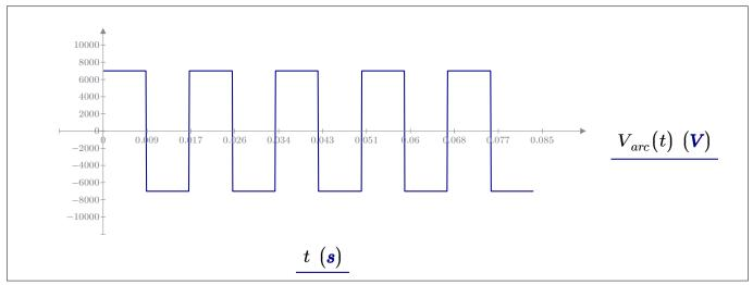
Figure 4. Typical waveform of arc voltage
