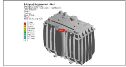
Figure 6. Non-linear static analysis
