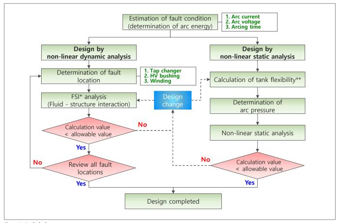
Figure 2. Tank design process
