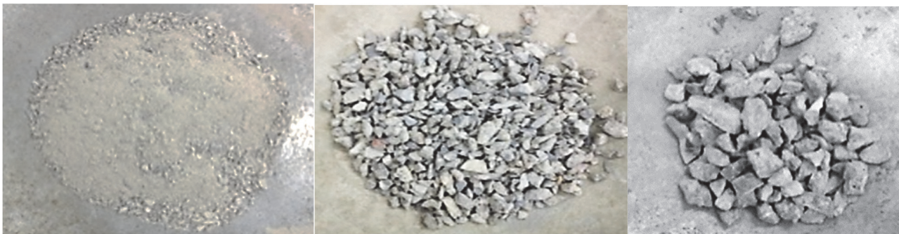
Figure 4: Produced recycled concrete aggregates fine and coarse.
