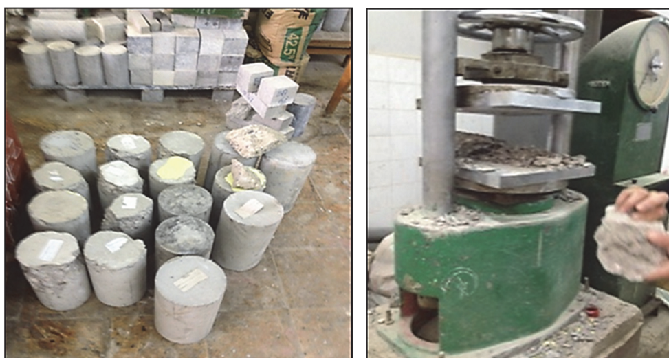
Figure 2: Test specimen crushed as concrete waste.
