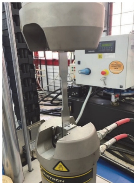
Figure 3: Experiment setup for cyclic test.
