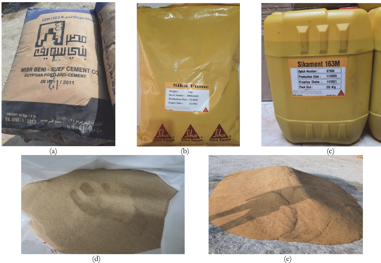
Figure 4: Material for UHPC mix. (a) Cement; (b) Silica fume; (c) Sikament 163M; (d) Micro sand; (e) Yellow sand.
