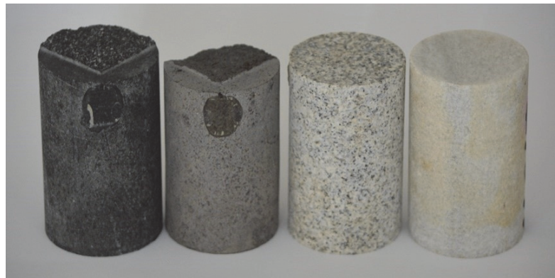
Figure 1: Rock specimens used for inclusion preparation after fracture tests (in order from left to right): amphibolite, basalt, granite and marble.
