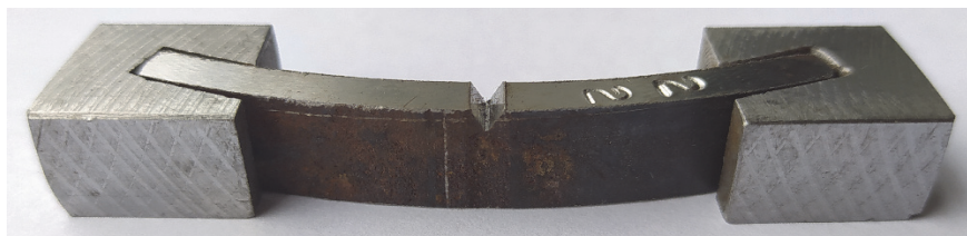
Figure 4: Specimen with tabs for the impact testing.
