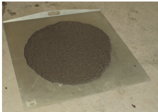
Figure 6: SCC mixture without segregation or bleeding.
