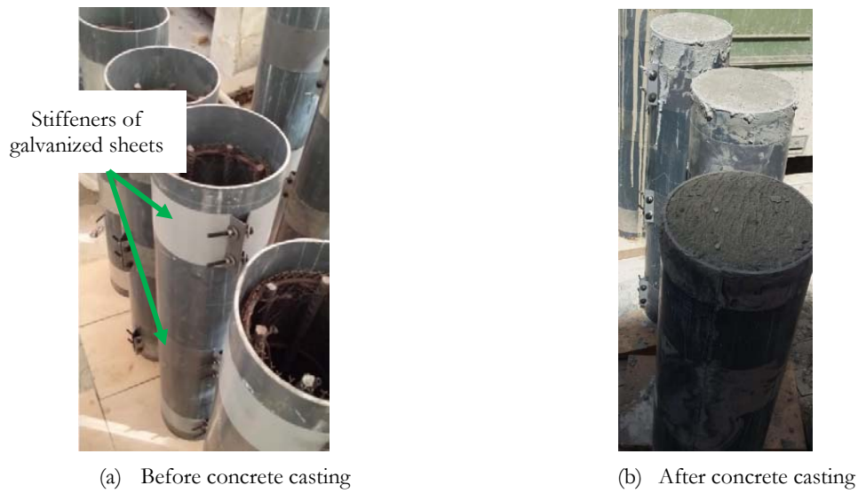
Figure 15: The used formworks in the current test.
