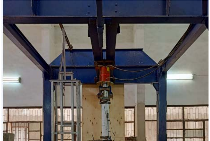
Figure 18: Loading configuration and test setup.
