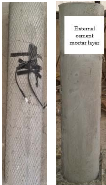
(a) Before using the cement mortar layer (b) After using the cement mortar layer
