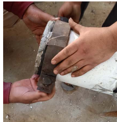
Figure 19: Steel collar at the ends.
