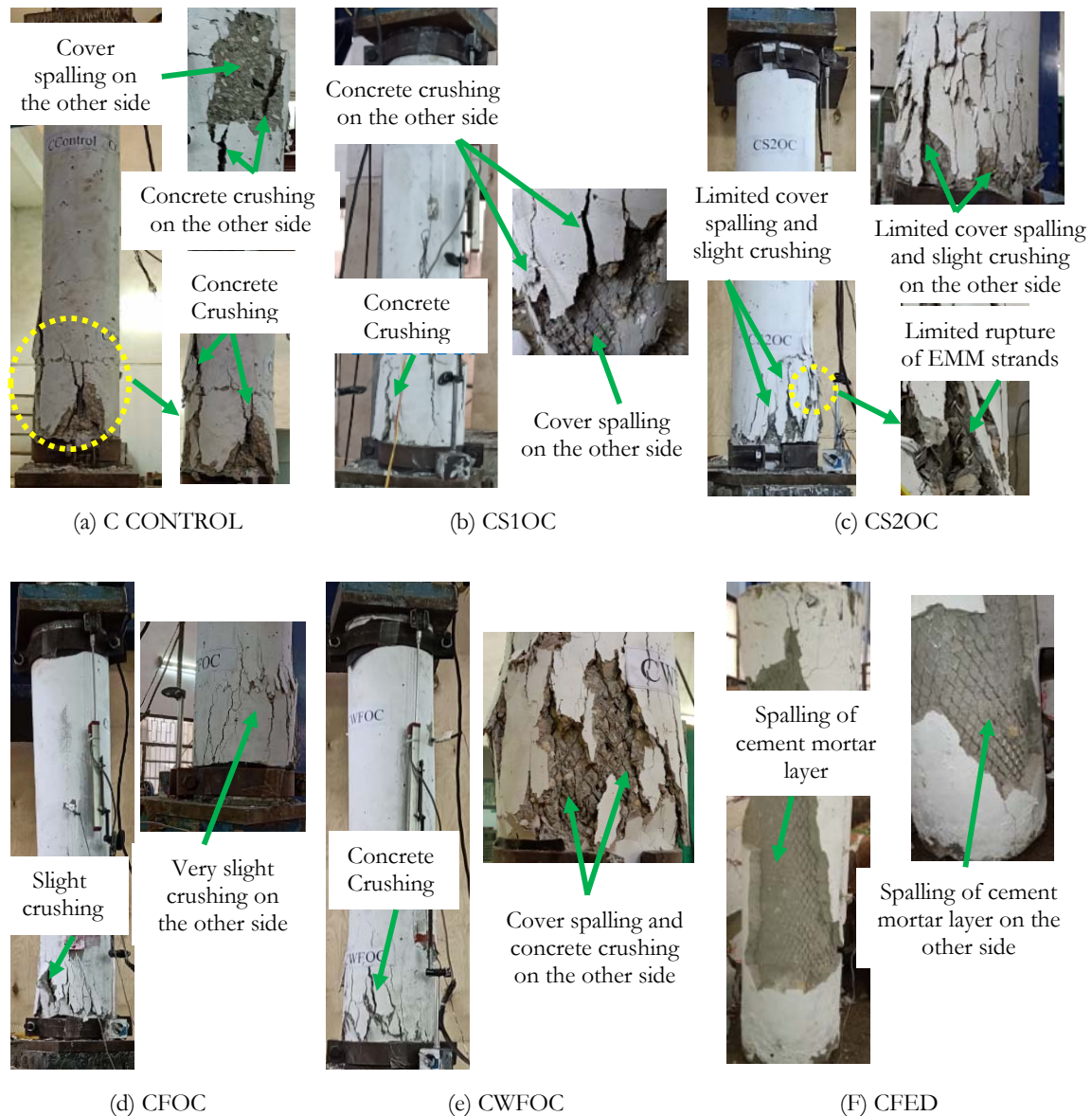
Figure 20: Crack patterns and failure modes of column specimens.
