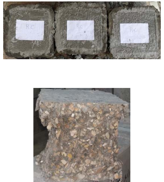
Figure 14: Cube specimens of compressive strength test.
