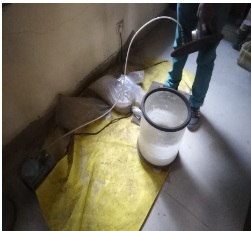
Fig-1 (a): Vacuum box and 1 (b): DC voltage system for RCPT Test
