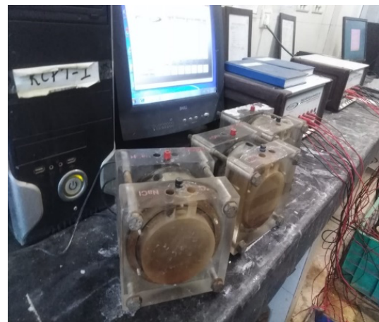
Fig-1 (a): Vacuum box and 1 (b): DC voltage system for RCPT Test
