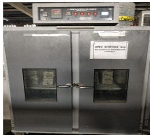
Fig-3: Carbonation Chamber for Accelerated Carbonation Test
