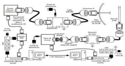
Fig 11. Components Interconnection.
