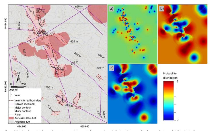
Figure 6. Updated geological map of research area, interpreted from non-linear indicator kriging; resulted from analysing probability distribution map of a) vein, b) andesitic tuff, and c) andesitic lithic tuff.
