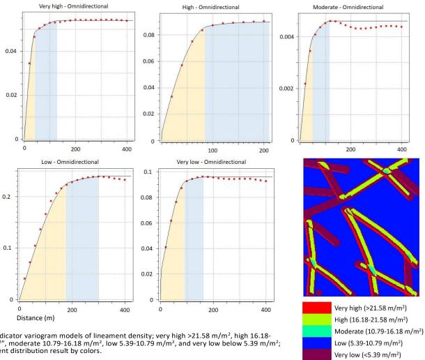
Figure 4. Indicator variogram models of lineament density; very high >21.58 m/m<sup>2</sup>, high 16.18-21.58 m/m<sup>2</sup>", moderate 10.79-16.18 m/m<sup>2</sup>, low 5.39-10.79 m/m<sup>2</sup>, and very low below 5.39 m/m<sup>2</sup>; the lineament distribution result by colors.
