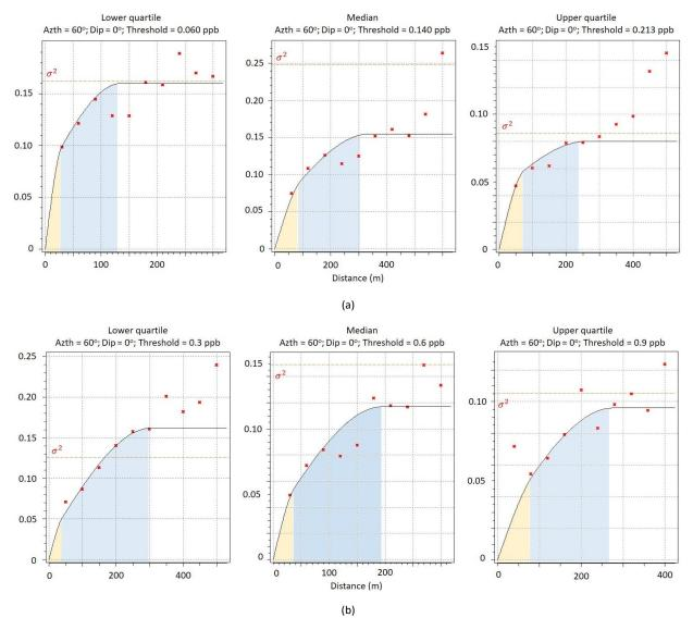
Figure 7. Indicator variogram models of continous data; (a) bismuth/Bi and (b) molybdenum/Mo, at each quartile thresholds.
