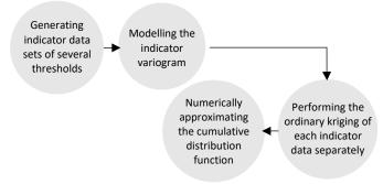
Figure 2. Non-linear Indicator Kriging algorithm.
