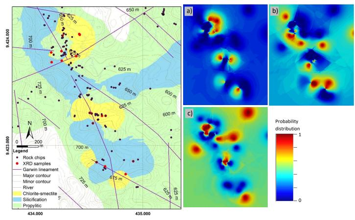
**Figure 5.** Interpreted lateral distribution of alteration map derived from non-linear indicator kriging; resulted from analysing probability distribution map of a) chlorite-smectite, b) propylitic, and c) silicification alterations.
