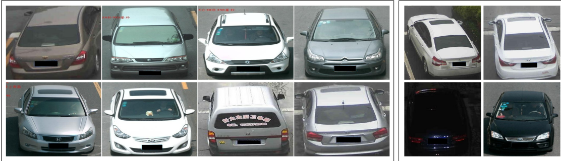
Figure 3.6: Qualitative evaluations of vehicle model classification. (Left) : Correctly classified vehicle images with large visual appearance similarity between different model classes. (Right) : Misclassified vehicle images due to extreme illumination conditions.
