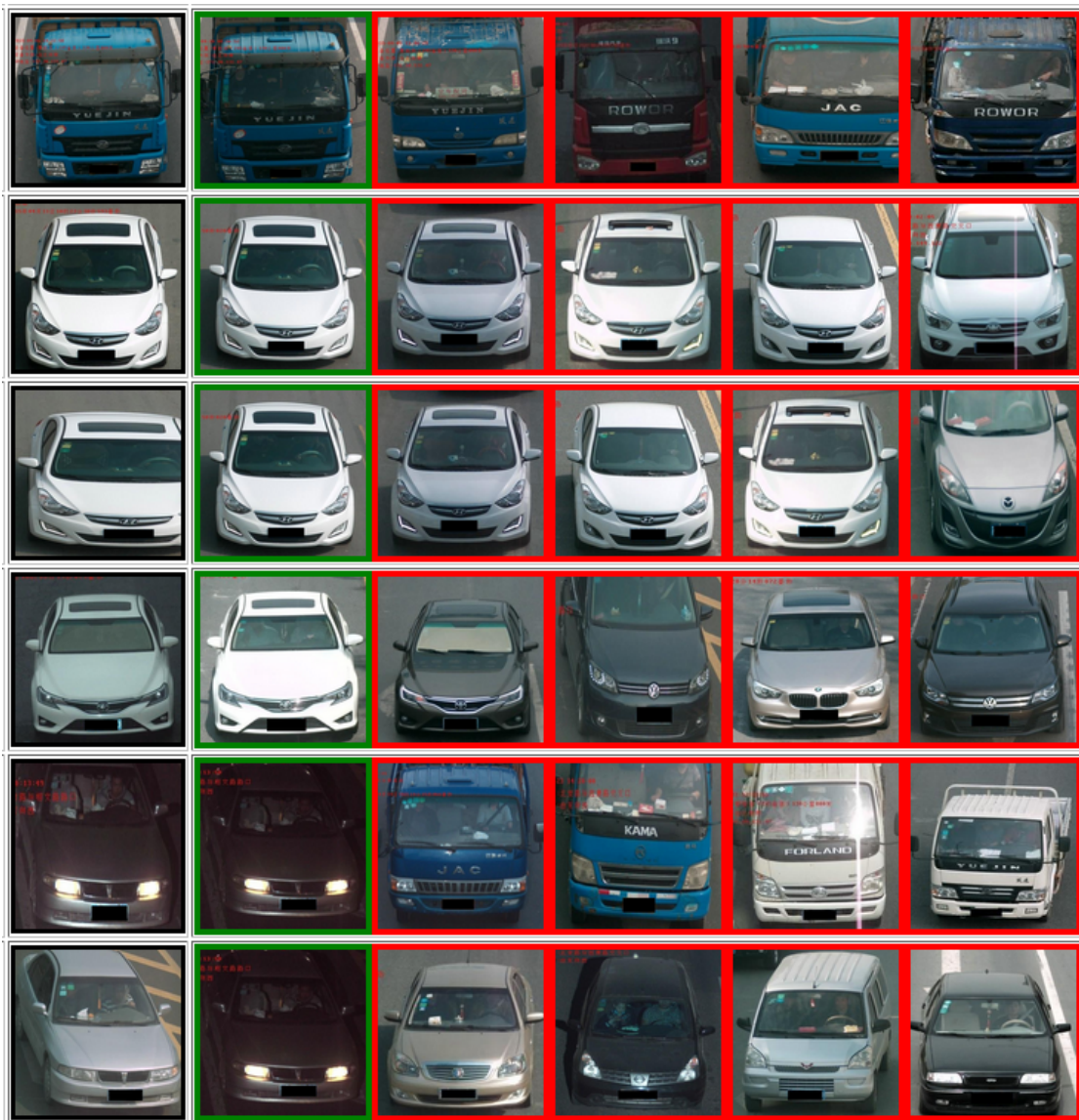
Figure 3.7: Highly successful Top-1 ranking examples. Left-most column is the probe image. Ranked images are ordered in ascending order by their distance from left to right. Green border shows same identity images, red border notes otherwise.(1 gallery image per ID)
