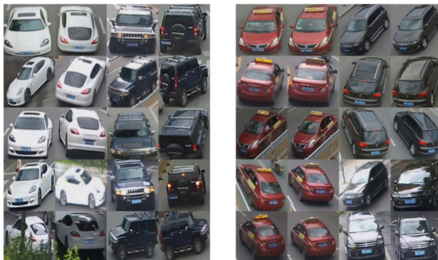
Figure 1.2: Inherent qualities of vehicles make vehicle re-ID an ill defined supervised learning problem where visually identical instances has different labels and same vehicle has captured at different location by different camera angle has dissimilar appearance. Examples images from VeRi-776[45] benchmark showcasing high intra-class variance and low inter-class variance.
