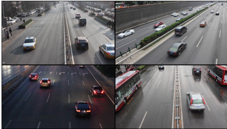
Figure 4.1: Realistic video frames from UA-DETRAC captured in uncontrolled environment showcasing: (a) common artefacts such as motion blur (b) low resolution with limited number plate visibility (c) different illumination due to time of day and changing weather conditions and time of day i.e. sunny, night, cloudy and rainy.
