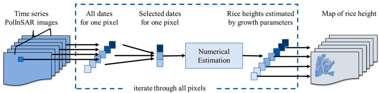
Figure 2. Flowchart of the height inversion implementation.
