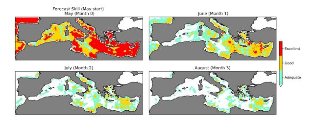
Figure 26. Anomaly Correlation Skill Score of Ocean Heat Content 0-40m in CMCC-SPS3.5 seasonal forecast system, over the period 1993-2016. It is an example of a new ocean variable being validated for Eurosea. It demonstrates the ability to make good predictions up to a season in advance in some parts of the Mediterranean Sea. Correlation score range for labels: adequate (0.4-0.6), good (0.6-0.8) & excellent (>0.8).
