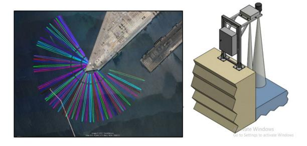
Figure 11. (a). Preferred jetty for installation of the Taranto tide gauge, showing a Fresnel zone (footprint for GNSS-IR) for one possible location (b) Proposed design of tide gauge framework and sea level instruments showing downward-projecting radar sensors
