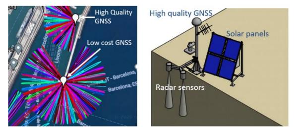
Figure 10. (a). Location for installation of the Barcelona tide gauge, with coloured radial lines showing a Fresnel zone (footprint for GNSS-IR) for the chosen locations of GNSS receivers (b) Proposed design of tide gauge framework and sea level instruments showing downward-projecting radar sensors and GNSS receiver.
