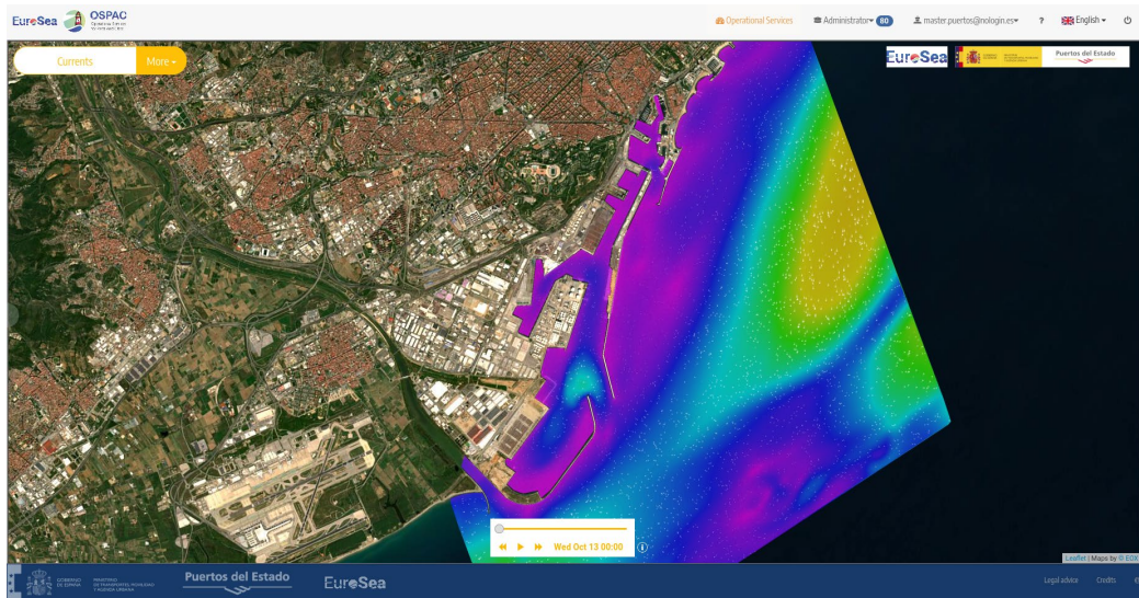
Figure 13. Forecasted surface currents at the Barcelona harbour, derived from a numerical model. The coloured areas denote the hourly-averaged surface current at the computational domain (70 m horizontal resolution).
