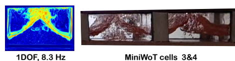
Figure 18. Average liquid surface location in 1DOF harmonic excitation tests [7] (left) and MiniWoT cells 3&4 sloshing pattern (right).
