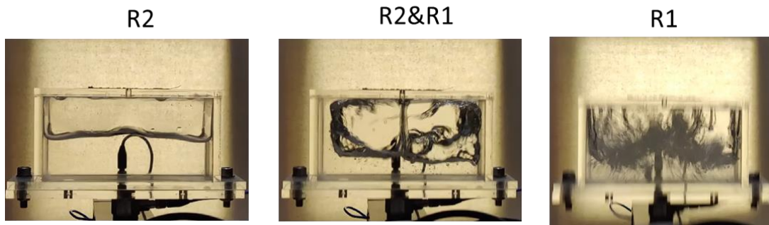
Figure 7. Different Sloshing regimes Excited During Harmonic Tests [4]
