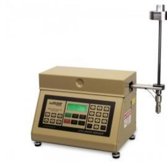
Scratching of coatings with controlled normal force
