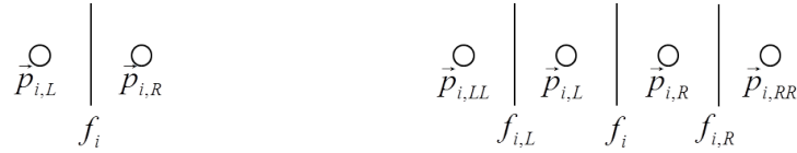
Figure 2.2: Identification of edge-points in an edge-based data structure (left) and of edge-faces in an enhanced edge-based data structure (right)
