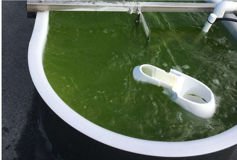
Figure 3. Effluent standpipe used for sample collection and to maintain the 30-cm pond depth. Mixing flow in the pond was counterclockwise.
