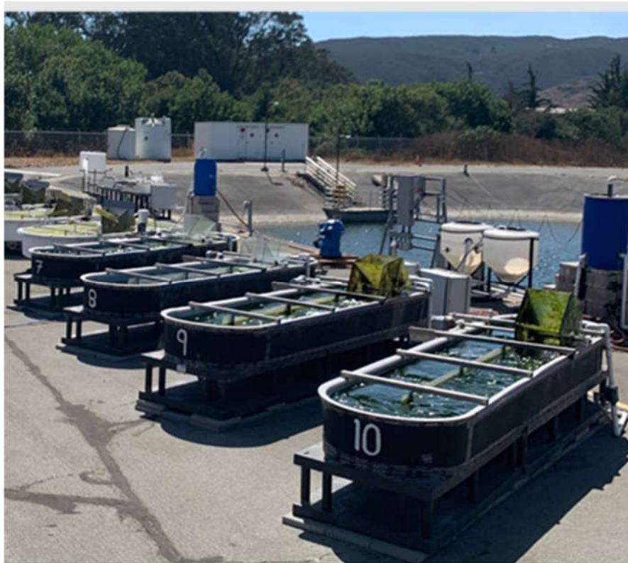
Figure 2. Paddle-wheel mixed raceway ponds used in the present study. (3.5-m 2 surface area, 0.3-m depth). Tribonema minus and the volunteer polyculture were each cultivated in duplicate ponds.
