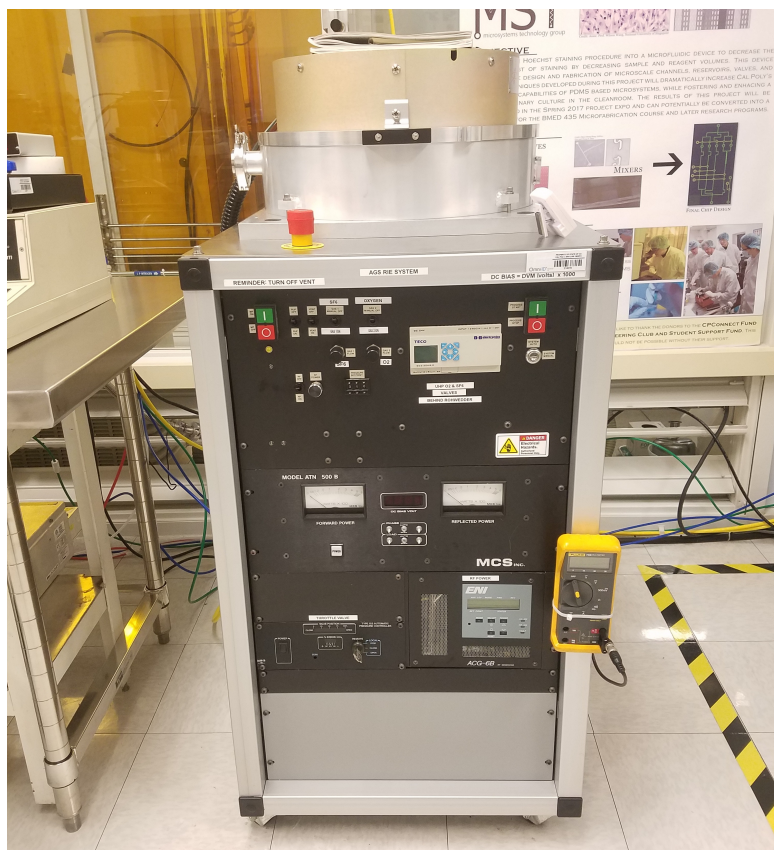
Figure 3.10: The AGS reactive ion etcher used to remove organic residue with an oxygen plasma.
