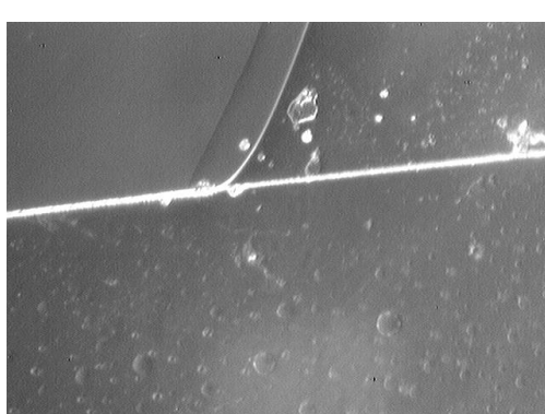
(d) Device delaminated after attempt to flush jammed sensor region.
