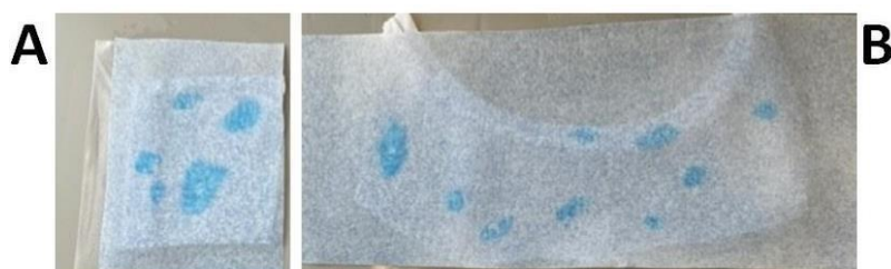
Figure S2: Phadebas paper test for the presence of amylase in saliva. A: image of right sleeve showing regions testing positive to amylase; B: entire neckline area showing regions testing positive to amylase. Positive areas were subsequently spotted with blood, then excised, extracted, and digested with trypsin prior to MALDI MSP analysis.
