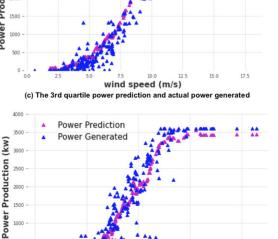
wind speed (m/s) (d) The 4th quartile power prediction and actual power generated FIGURE 11. The power prediction and actual power generated for each quarter Q1, Q2, Q3,and Q4 from left to right using kNN regression.
