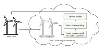
FIGURE 3. A cloud-based framework to model the wind farm using digital twins technology and predictive modeling to forecast the generated power.
