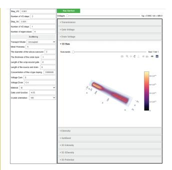
One of many Sim2l implemented simulations, showing a configurable and interactable silicon nanowire with the 3D bias display, with additional options to analyze potential profile, electron density, and more.
