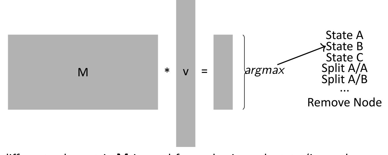
A different rule matrix **M** is used for nodes in each state (ie. a three-state system would have three different rule matrices).
