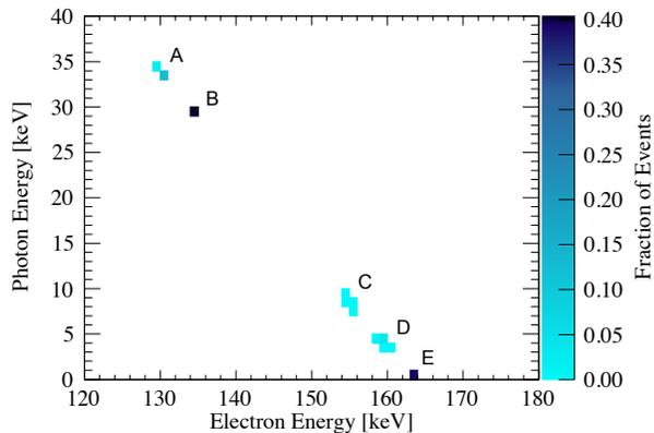
FIG. 16. Photon energy versus electron energy for  $^{131m}\text{Xe}$  decays. The sum of the two always gives 163.93 keV total energy deposition. The colour scheme shows the fraction of events in a particular region. Labels A – E show different populations formed by various combinations of conversion electrons, Auger electrons and X-rays.
