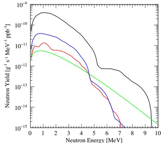
FIG. 10. Neutron spectra from  $(\alpha, n)$  reaction from uranium decay chains in equilibrium ( $^{238}\text{U}$  and  $^{235}\text{U}$  are combined together) in 3 materials: black - PTFE ( $\text{C}_2\text{F}_4$ ), blue - ceramics ( $\text{Al}_2\text{O}_3$ ), red - titanium. The green curve shows the spectrum from spontaneous fission (same for all materials).
