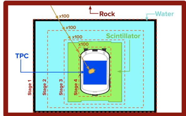
FIG. 6. A schematic drawing of the event biasing method implemented into BACCARAT allowing the simulations of the cavern rock  $\gamma$ -rays. The relative dimensions of the cavern, water tank, LS veto, and TPC are not to scale.
