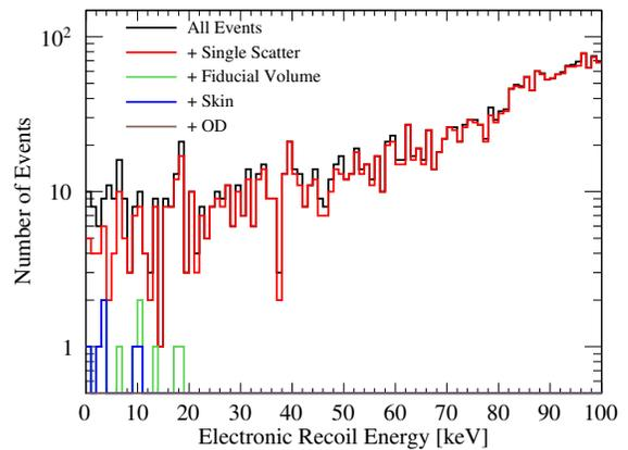
FIG. 14. Energy spectra of all muon-induced events in the liquid xenon TPC. The spectra are shown for events surviving each of the analysis cuts applied consecutively.  $2.3 \times 10^8$  muons corresponding to approximately 120 years of live time were simulated in LUXSim and analysed applying standard background rejection cuts. No event survived all cuts in the 6 – 30 keV<sub>nr</sub> range.
