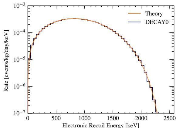
FIG. 19. Summed electron recoil energy spectrum of the  $^{136}\text{Xe}$   $2\nu\beta\beta$  decay. Theoretical curve (orange) from [82] is superimposed on the simulated histogram (black) from the DECAY0 generator [83].
