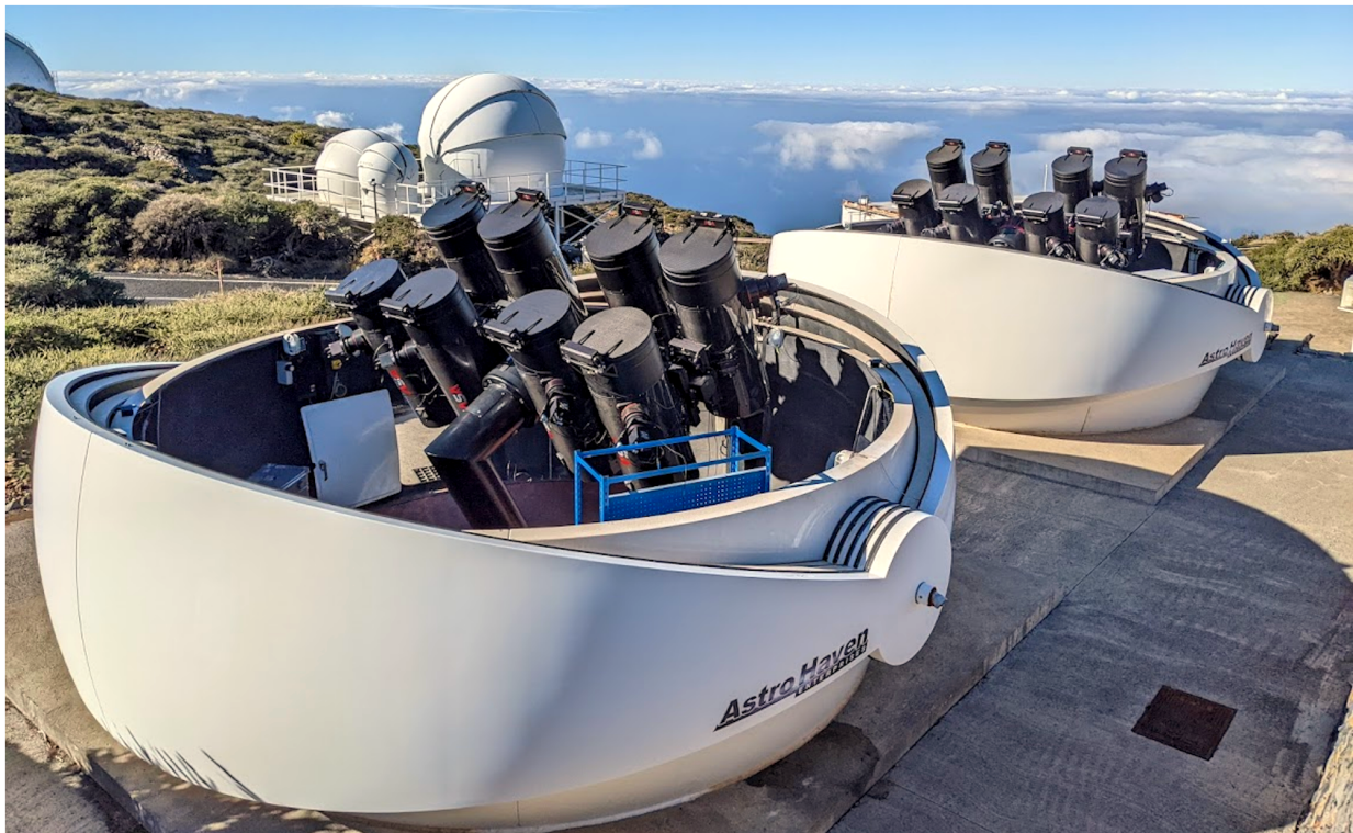
Figure 3. The complete GOTO-North node as of 2021. Each dome hosts a single mount with eight unit telescopes.
