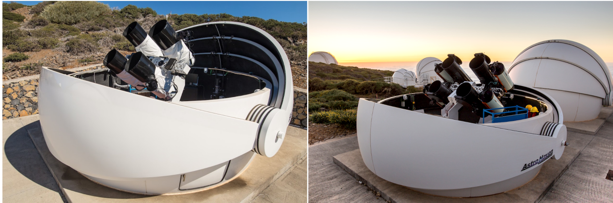
Figure 2. The original GOTO prototype in the dome on La Palma. On the left the initial four unit telescopes are shown in 2019, attached to the prototype mount. On the right in 2020 the prototype unit telescopes have been replaced with the new ASA design, alongside four temporary Celestron RASAs on the outside of the array.
