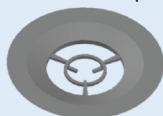
Figure 2 – A 3D rendering of the sample holder that is held in place at the bottom of the vessel by magnets (see Figure 1).
