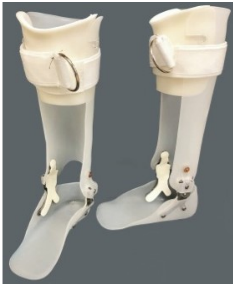
Figure 4-5: Articulated AFO with a hinge at the ankle. The axis of the joint is aligned as closely as possible to the bending axis of the physiological ankle joint. This should reduce torque and shear forces. Reproduced with permission of the copyright holder, Elsevier.
