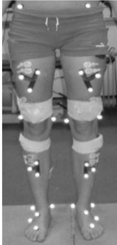
Figure 9-3: Marker set up for the BBImperial model with clusters on the thigh and tibia (Duffell, 2014). Markers are placed on the Anterior superior iliac spines (ASIS) bilaterally, the Posterior superior iliac spines (PSIS) bilaterally, clusters on the thigh shanks, medial and lateral femoral condyles bilaterally, tibia shanks bilaterally, medial and lateral malleoli bilaterally, over the 2 nd metatarsal, 5 th metatarsal, and the heel, bilaterally. Reproduced with permission of the copyright holder, Sage.
