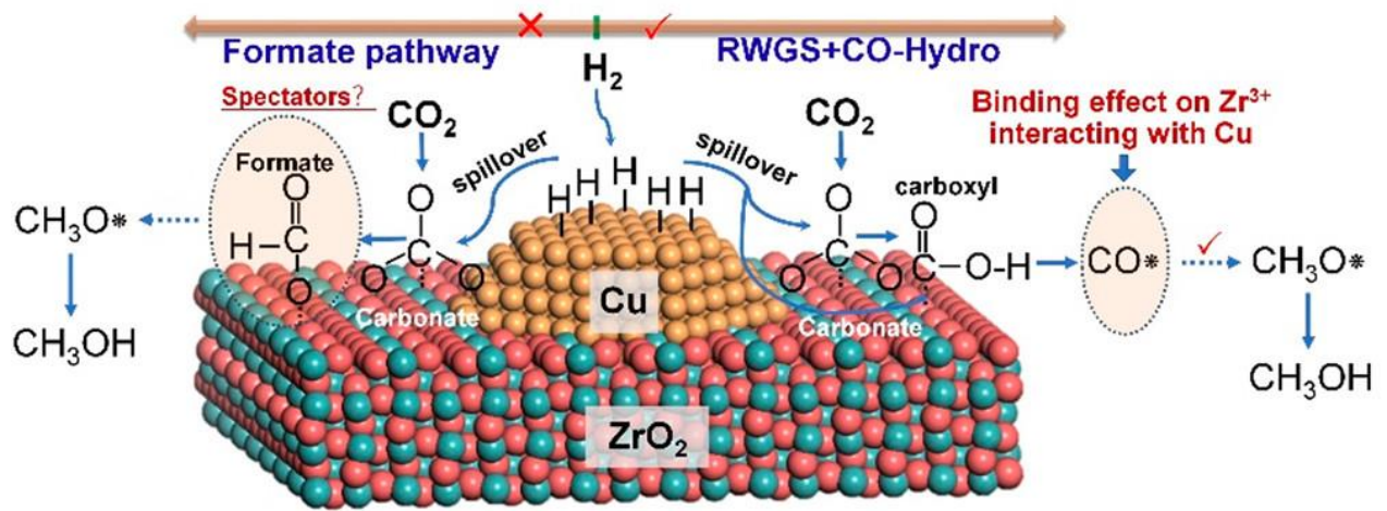
Figure 1.2 - Possible reaction pathways and active sites of CO 2 hydrogenation to CH 3 OH over the Cu/ZrO 2 . (78)
